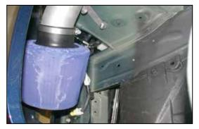
31. Slide the K&N<sup>®</sup> air filter onto the K&N<sup>®</sup> cold air tube and secure with the provided hose clamp as shown.
