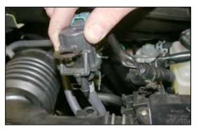
6. Using a flat blade screwdriver pry up the vacuum switching valve from the stock intake tube as shown.
