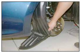
16. Remove four screws and three plastic rivets, then, pull the inner fender valance downward as shown.
