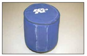
30. Slide the Drycharger<sup>®</sup> onto the K&N<sup>®</sup> air filter as shown above
