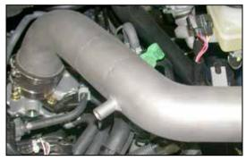
22. Slide the  $K\&N^{\otimes}$  intake tube into the silicone hose on the throttle body as shown.
