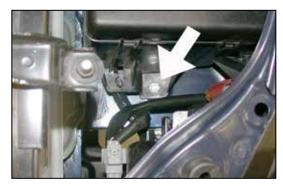
28. Install the provided hex bolt into the fuse box mount from the previous step as shown.
