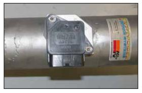
20. Install the mass air sensor into the K&N<sup>®</sup> intake tube and secure with the provided hardware as shown.
