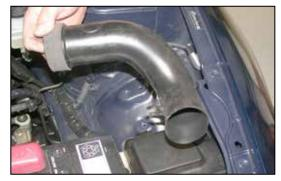
12. Remove the air inlet duct as shown.
