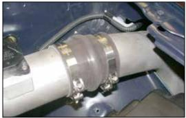
26. Slide the K&N<sup>®</sup> cold air tube through the inner fender from underneath the vehicle and insert the tube into the silicone hump hose as shown above. **NOTE:** Before installing the intake tube, inspect the inside of the tube for any debris, then clean the inside out with water and a towel. Inspect the tube one more time before proceeding to the next step.
