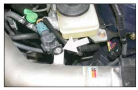
24. Secure the vacuum switching valve to the bracket on the K&N<sup>®</sup> intake tube using the provided hardware as shown.
