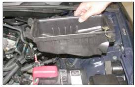
11. Remove the lower air cleaner assembly as shown.
