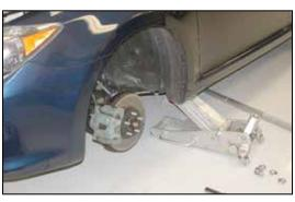
15. Raise the vehicle up and support it with jack stands, then, remove the front tire as shown.
