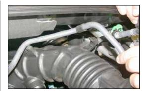
7. Unclip the vent hose from the stock intake tube as shown.
