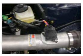
36. Reconnect the mass air sensor electrical connection as shown.
