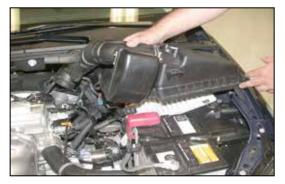
9. Depress the spring clamp on the throttle body, then, remove the complete upper air cleaner assembly as shown.
