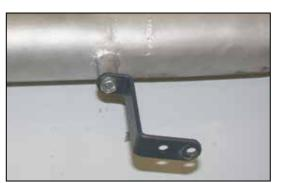
19. Install the provided bracket onto the K&N<sup>®</sup> intake tube and secure with the provided hardware.
