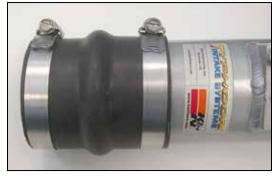
21. Install the provided silicone hump hose and hose clamps onto the  $K\&N^{\circledast}$  intake tube and secure as shown.
