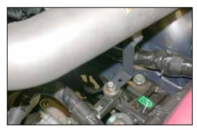
23. Secure the bracket to the rubber mounted stud using the provided hardware but do not tighten at this time.
