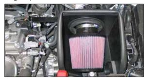
20. Install the K&N<sup>®</sup> air filter and secure with the
