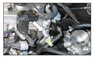
10. Remove the fuel rail mounting bolt shown. **NOTE: This bolt will be re-used.**
