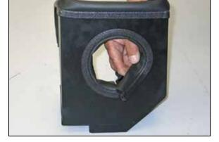
15. Install the short edge trim onto the heat shield as shown. **NOTE: Some trimming of the edge trim may be necessary.**  provided hose clamp.
