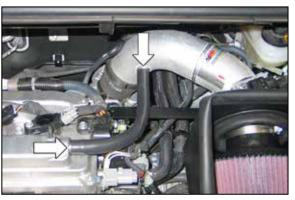
21. Install the provided crank case vent hose as shown.
