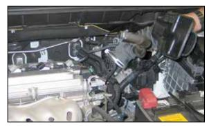
7. Disconnect the crank case vent hose from the valve cover. Loosen the spring clamp that secures the intake tube to the throttle body and remove the stock intake tube from the vehicle.
