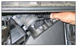
3. Depress the locking tab on the mass air sensor electrical connection, then disconnect the mass air sensor electrical connector.
