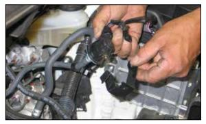
9. Remove the screw that secures the EVAP mounting bracket, then remove the bracket as shown.
