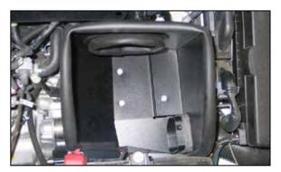
16. Install the heat shield assembly and secure with the provided hardware. NOTE: The fresh air supply tube is to be installed into the heat shield.
