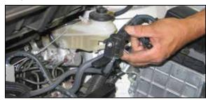
13. Install the provided EVAP bracket onto the EVAP solenoid with the provided hardware.
