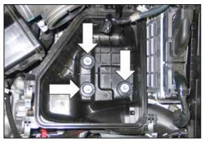
6. Remove the three bolts that secure the lower air box. Then, un-clip the wiring harness and remove the lower air box from the vehicle.
