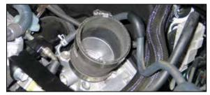
12. Install silicone step hose (#08713) onto the throttle body and secure with the provided hose clamp.
