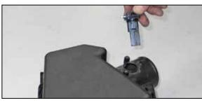
17. Remove the two screws that secure the mass air sensor to the stock air box. Then, remove the mass air sensor as shown.
