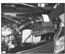
6. Release the two upper air box mounting clips and then remove the upper air box and intake tube assembly as shown.
