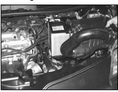
8. Release the mass air sensor wiring harness from the lower air box and then remove the lower air box from the vehicle as shown.
