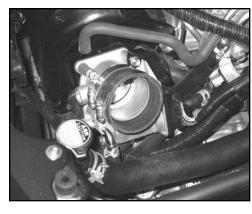
20. Install the supplied silicone hose (084014) onto the throttle body and secure it with the provided hose clamp.
