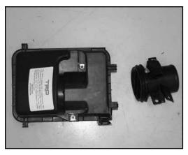
12. Remove the two bolts that secure the mass air sensor to the upper air box and then remove the mass air sensor as shown.
