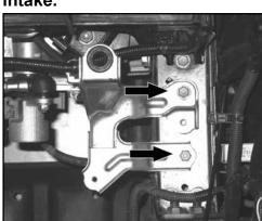
9. Remove the two bolts that secure the air box mounting bracket.
