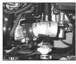
21. Install the K&N® intake tube into the silicone hose on the throttle body and align with the mounting bracket installed during step #19. Secure the intake tube with the provided hardware.
