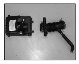
11. Loosen the hose clamp that secures the stock intake hose to the mass air sensor. Disconnect the intake hose from the mass air sensor as shown.
