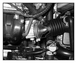
5. Loosen the hose clamp which secures the stock intake hose to the throttle body.
