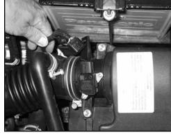
3. Depress the locking tab on the mass air sensor electrical connection and disconnect the electrical connector from the mass air sensor. Unhook the mass air sensor wiring harness from the mounting tabs on the air box.
