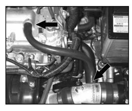
25. Install the supplied silicone hose onto the fitting on the valve cover. Attach the other end to the vent port on the K&N® intake tube.
