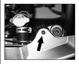
15. Remove the factory bumper cover mounting pin from the core support as shown.
