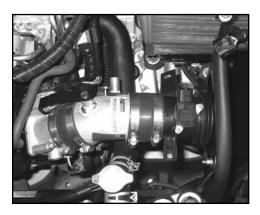
23. Pass the mass air sensor assembly through the heat shield and secure it to the intake tube with the provided hose clamp as shown.
