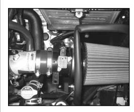
26. Reconnect the mass air sensor electrical connection and secure the mass air sensor wiring harness to the mass air sensor housing.
