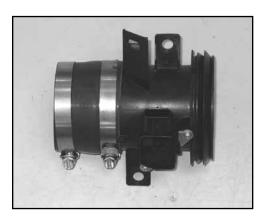
22. Install the remaining silicone hose (084014) onto the mass air sensor and secure it with the provided hose clamp.
