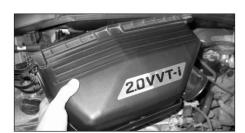
3. Unclip and remove the air box lid from the vehicle as shown.
