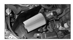
22. Align the new intake tube for maximum clearance; now firmly tighten all clamps, nuts and bolts.
