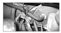
27. Fit the vacuum switch onto the big vacuum hose as shown, using a cable tie supplied.
