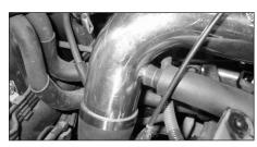
24. Mount the breather hose onto the new intake tube using the original hose clamp as shown
