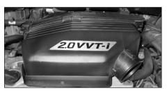
25. Refit the complete air box back onto the engine as shown.
