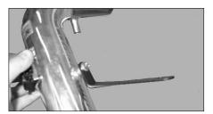
18. Mount the "L" bracket onto the new intake tube using the hardware supplied.
