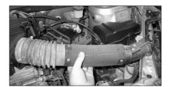
2. Unclip and remove the air inlet duct from the vehicle as shown.
