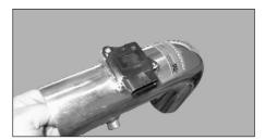
13. Install the MAS into the intake tube using the provided hardware. **NOTE**: Before installing clean the inside of out with water and a towel!
