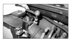
8. Loosen the hose clamps at the throttle body and at the air box.
