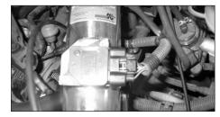
23. Re-connect the mass air sensor electrical connection as shown.
