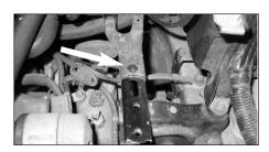
15. Remove the bolt that secure the wire loom bracket to the gear box mounting bracket as shown
