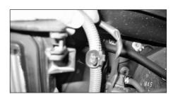
4. Unclip the wire harness from the air box base as shown.
