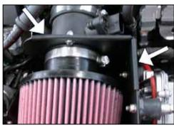
37. Using the supplied edge trim, cut to size and fit over the heat shield as shown.
