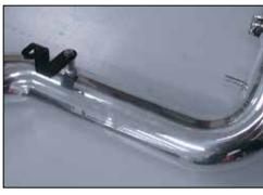
35. Install the "Z" bracket to the intake tube as shown.
