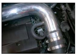
44. Route the hose underneath the intake tube and connect it to the vent tube on the intake tube as shown.
