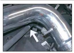
41. Insert the hose mender into the stock EVAP recirculation line as shown.
