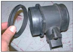
20. Remove the mass air sensor O-ring from the mass air sensor.
