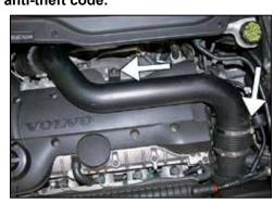
2. Remove the two bolts that secure the stock intake tube.
