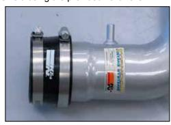
34. Install the silicone hose and provided hose clamps to the K&N® intake tube.
