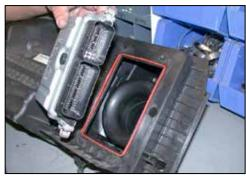
19. Remove the four bolts that secure the ECM to the air box using a T30 torx.
