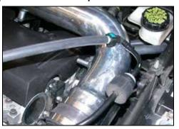
43. Insert the carbon filter vacuum hose onto the stock crank case hose as shown.
