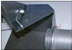
22. Install the "L" bracket onto the heat shield and secure it with the provided hardware.
