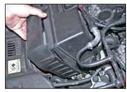
8. Lift and remove the plastic ECM cover from the air box.
