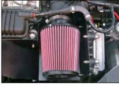
36. Secure the K&N® air filter onto the stock mass air sensor using the provided hose clamp.
