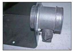
21. Install the mass air sensor onto the heat shield and secure it with the provided hardware.
