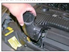
14. Pull upwards to remove the lower air inlet duct from the air box as shown.
