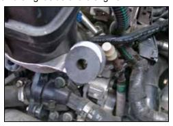
28. Install the threaded insert into the air box mounting hole from step 26.
