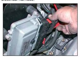
31. Re-connect the two electrical wiring harness to the ECM.
