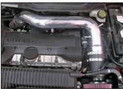
38. Install the K&N® intake tube into the stock intake hose, attaching the other end onto the mass air sensor. Secure the intake tube to the stock hose with the stock hose clamp and secure the intake tube to the mass air sensor with the provided hose clamp.
