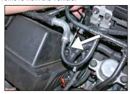
7. Remove the bolt that secures the main wiring harness to the air box, then unclip the harness from the air box.
