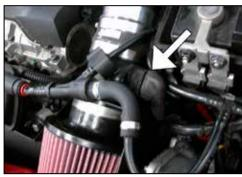
48. Reconnect the mass air sensor electrical connection.
