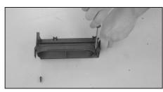
9. Using a small screw driver remove the two clip nuts from the lower fresh air duct as shown.
