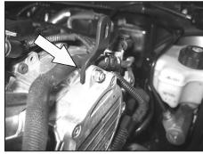
19. Install the tube mounting bracket (010038) onto the left side of the engine cylinder head as shown and secure with the provided hardware.
