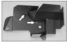
12. Install heat shield #07350 onto heat shield #07351 and secure with provided hardware.
