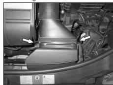
3. Remove the two screws shown that secure the fresh air tube to the fresh air duct.
