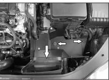
16. Install the heat shield assembly and fresh air duct into the vehicle so that the heat shield mounting grommets are snapped onto the mounting studs and the fresh air duct snaps into the fresh air supply tube, secure the duct and heat shield with the provided hardware.
