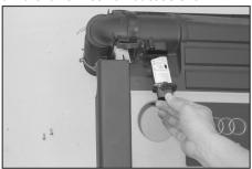
10. Remove the two screws that secure the mass air sensor to the stock air filter housing and then remove the mass air sensor as shown.
