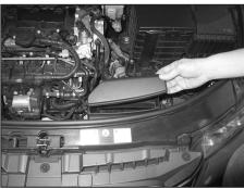
7. Remove the upper fresh air duct cover as shown.
