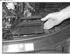
8. Unsnap and remove the lower fresh air duct as shown.
