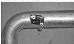
11. Install the mass air sensor into the  $K\&N^{\circledast}$  intake tube with the provided hardware.
