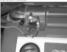
2. Disconnect the mass air sensor electrical connection and unhook the mass air sensor wiring from the engine cover.
