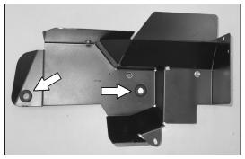
14. Install the two heat shield mounting grommets into the mounting holes as shown.
