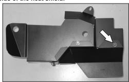
13. Install the third bolt to secure heat shield #07350 to heat shield #07351 from the bottom side as shown. Completely tighten all three bolts.
