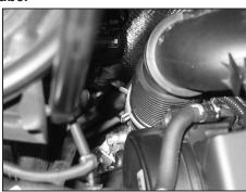
5. Using pliers, release the spring clamp that secures the intake to the intake inlet. Then unhook the intake tube from the inlet.
