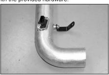
11a. Install the tube mounting bracket (070107) onto the K&N® intake tube and secure with the provided hardware.
