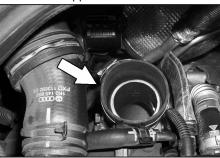
18. Install the provided silicone hose (084016) onto the turbo inlet and secure with the provided hose clamp.
