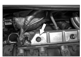
6a. Remove the airbox mounting stud shown
