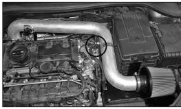
21. Install the K&N® intake tube into the silicone hose at the turbo inlet and align with the bracket installed during step 19. Secure the bracket attached to the intake tube (070107) to the airbox mounting location. Secure the intake tube with the provided hose clamp and hardware.
