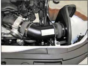
18. Install the K&N<sup>®</sup> intake tube into the silicone hump hose and then into the into the silicone step hose at the throttle body. Align the intake tube and heat shield for proper fit and then secure the intake tube with the provided hose clamps and the heat shield bracket with the factory air box retaining bolt removed in an earlier step.
