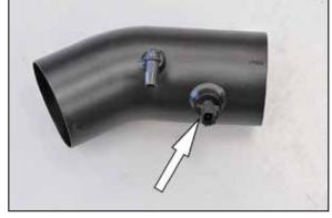
17. Install the inlet air temperature sensor into the  $K\&N^{\mbox{\tiny B}}$  intake tube as shown.
