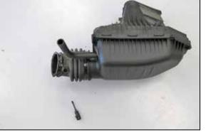
16. Remove the inlet air temperature sensor from the factory intake tube as shown.
