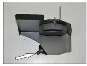
10. Install the provided inserted nut onto the heat shield as shown and secure with the provided hardware.
