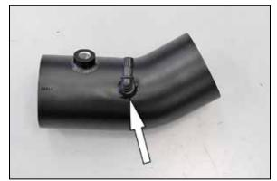
15. Install the provided  $90^{\circ}$  vent fitting into the K&N<sup>®</sup> intake tube as shown.
