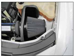
24. Install the K&N<sup>®</sup> air filter and secure with the provided hose clamp.
