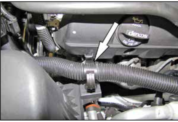
7. Open the clamp securing the sound tube to the air filter housing.
