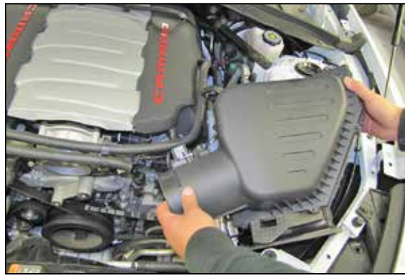
12. Lift up the air filter housing to dislodge it from the mounting grommets and then remove it from the vehicle.
