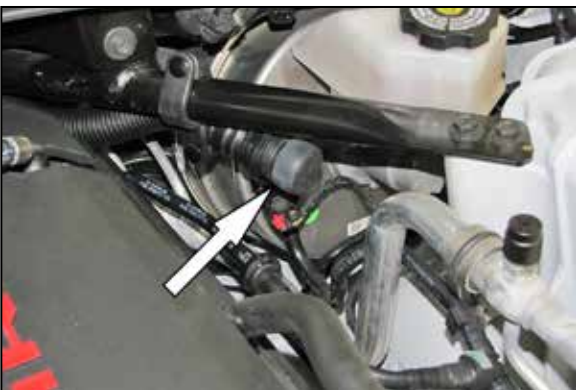
11. Install the cap assembly into the remaining sound tube.
