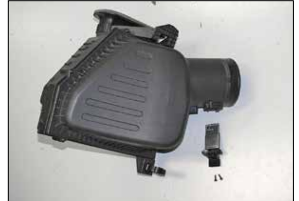
18. Remove the mass air sensor from the factory air filter housing.
