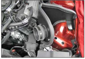
17. Install the provided silicone hump hose (08699) onto the filter adapter and secure with the provided hose clamp.
