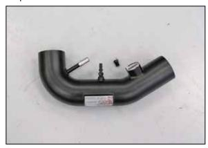
19. On vehicles equipped with an EVAP vent line, install the provided quick disconnect fitting into the K&N<sup>®</sup> intake tube. On vehicles not equipped with the EVAP vent line, install the provided 1/4npt plug into the K&N<sup>®</sup> intake tube.
