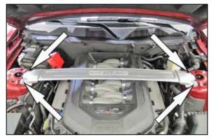
2. On vehicles equipped with a strut tower brace, remove the four nuts that secure the brace and then remove the brace from the vehicle.
