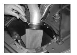
26. Install the K&N<sup>®</sup> air filter and secure with the provided hose clamp as shown. NOTE: Drycharger<sup>®</sup> air filter wrap; part # RC-3690DK is available to purchase separately. To learn more about Drycharger<sup>®</sup> filter wraps or look up color availability please visit http://www.knfilters.com.
