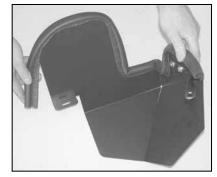
12. Install the provided edge trim onto the heat shield. Trim if necessary.
