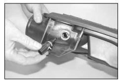
17. Twist the temp sensor counter clockwise to unlock and remove the temp sensor from the resonator.
