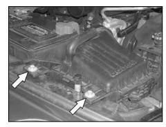
4. Remove the two air box retaining bolts.
