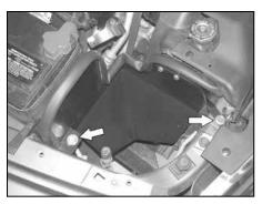
15. Install the heat shield assembly and secure the mounting bracket to the radiator core support with original bolt removed in step #13. Secure the rear of the heat shield to the 3/8" threaded insert with the provided hardware.
