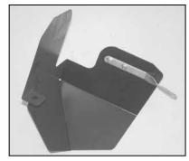
11. Install the heat shield bracket (07197) onto the heat shield with the provided hardware.
