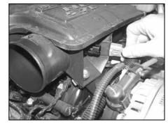
7. Depress the locking tab on the air temp sensor and disconnect its electrical connection. **NOTE: Take care when handling the temp sensor as it is very fragile.**
