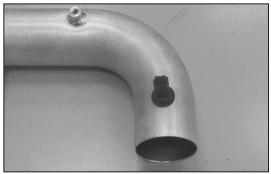
8. Install the air temperature sensor into the grommet installed into the K&N® intake tube during step #6.
