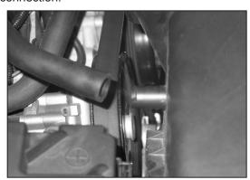
3. Disconnect the crankcase vent hose from the stock intake tube as shown.
