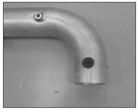
6. Install the supplied grommet into the hole in the  $K\&N^{\odot}$  intake tube as shown.
