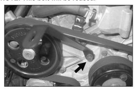
11. Install the supplied tube mounting bracket (26653) onto the engine and secure with the bolt removed in step #10.
