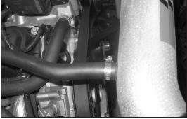
20. Connect the crankcase vent hose to the K&N<sup>®</sup> intake tube and secure with the provided hose clamp as shown.
