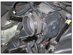
21. Install the provided silicone hose (08690) onto the throttle body and secure with the provided hose clamp.
