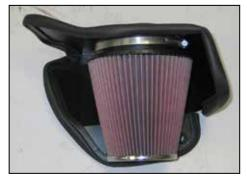
15. Install the K&N<sup>®</sup> air filter onto the filter adapter and secure with the provided hose clamp. NOTE: Drycharger<sup>®</sup> air filter wrap; part # RF-1041DK is available to purchase separately. To learn more about Drycharger<sup>®</sup> filter wraps or look up color availability please visit http://www.knfilters.com<sup>®</sup>. 20. Install the provided hump hose (084057) onto to the filter adapter and secure with the provided hose clamp.
