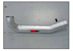
19. Install the provided ¼ npt vent fitting into the K&N<sup>®</sup> intake tube #27447 as shown. NOTE: Plastic NPT fittings are easy to cross thread. Install the vent fitting "hand" tight, then turn it two complete turns with a wrench.
