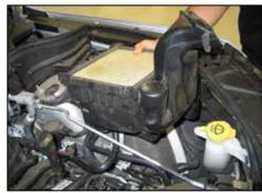
2. Lift up the engine cover to unhook it from the mounting grommets and then remove the engine cover from the engine.
