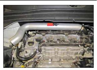
17. Install the K&N® intake tube assembly into the coupling hose and align the bracket with the mounting lug on the valve cover. Tighten the hose clamps but do not secure the bracket to the valve cover.
