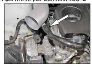
20. Connect the crank case vent hose to the fitting installed into the  $K\&N^{\mbox{\scriptsize 0}}$  intake tube.
