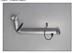
16. Connect the inlet air temperature extension harness provided to the sensor as shown.
