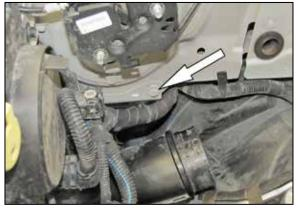
21. Remove the inner fender bolt shown.
