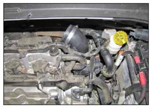
8. Install the provided coupling hose (08489) onto the throttle body with the hose clamps but do not tighten at this time.
