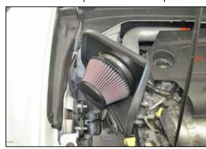
28. Install the filter assembly onto the K&N® intake tube and adjust for best fit and then secure with the provided hose clamp.
