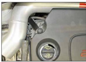
19. Install the engine cover and align the tube mounting bracket then secure the bracket and engine cover using the factory bolt from step #2.
