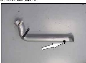
15. Remove the O-Ring from the sensor and then install the sensor into the grommet installed into the  $K\&N^{@}$  intake tube.
