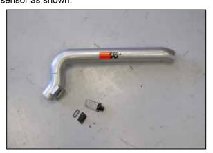
10. On vehicles equipped with a mass air sensor, install the sensor into the K&N® intake tube and secure with the provided hardware. On vehicles that are not equipped with a humidity sensor, install the provided gasket onto the block off and then install the block off into the K&N® intake tube and secure with the provided hardware.
