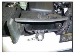
4. Remove the bolt shown that secures the fresh air intake duct to the fender, then lift and remove the complete intake system from the vehicle. NOTE: The factory mounting grommets should remain in the vehicle. NOTE: K&N Engineering, Inc., recommends that customers do not discard factory air intake.
