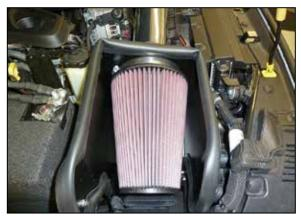
14. Install the K&N<sup>®</sup> air filter and secure with the provided hose clamp.
