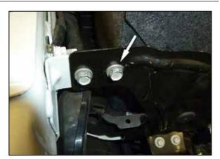
5. Remove the inner bolt that attaches fender bracket to the fender.
