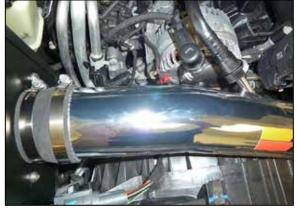
13. Connect the crank case vent line to the  $K\&N^{\otimes}$  intake tube.
