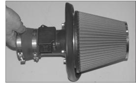
22. Assemble the K&N $^{\!0}$  air filter onto the heat shield assembly as shown.
