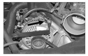
13. Remove the upper alternator bolt and harness clip, and then secure the tube-mounting bracket (070018) to the alternator with the removed bolt.
