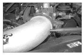
16. On vehicles that come equipped with a second vent line, line up the vent hose on the intake tube and make a mark on the intake tube for drilling.
