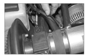
23. Install the heat shield assembly onto the K&N $^{\! \otimes }$  intake tube and tighten the hose clamp as shown.
