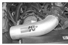
17. Re-install the K&N® intake tube onto the throttle body and mounting bracket and then secure with the provided hose clamp and hardware.
