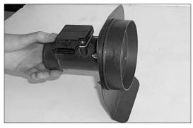
9. Assemble the mass air adapter, gaskets, heat shield and mass air sensor as shown.
