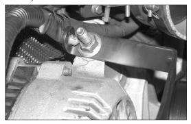
14. Push the wire harness-retaining clip into the hole on the tube-mounting bracket as shown.
