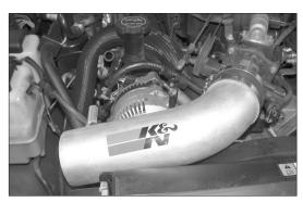
15. Install the K&N® intake tube onto the throttle body and line it up with the tube-mounting bracket, then secure with the hose clamp and hardware provided.
