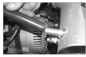
20. Install the crank case vent hose assembly into the 90° fitting at the valve cover and then connect to the vent fitting on the K&N® intake tube as shown.
