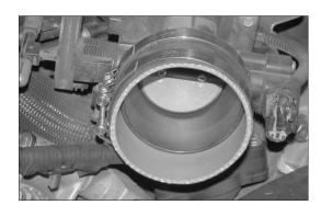
12. Install the silicone hose (08630) and the hose clamps onto the throttle body as shown.
