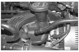
18. Remove the factory plastic crank case vent hose from the 90° elbow on the valve cover as shown.
