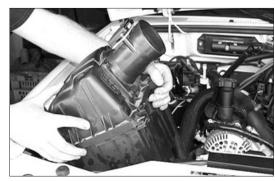
7. Using a screwdriver, pry up the bottom of the air cleaner to release the air cleaner from the stock grommets, then remove the air cleaner assembly as shown.
