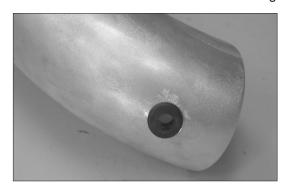
16a. After marking the intake tube, remove the tube from the vehicle and drill a 5/8" hole into the intake tube then install the provided grommet as shown.
