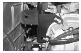
25. Install the tube mounting bracket onto the valve cover using the factory bolts. Do not completely tighten the bolts at this time.
