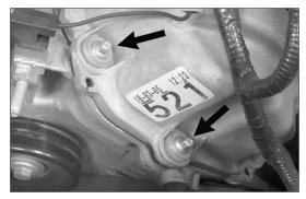
23. Remove the two valve cover mounting bolts shown.
