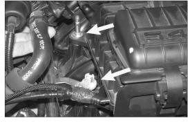
5. Pull up on the heater control valve and wiring harness mounting clips to unhook them from the air box mounting studs as shown.
