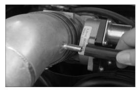
30. Connect the factory brake booster vent hose to the K&N $^{\circ}$  intake tube and secure with the provided hose clamp.
