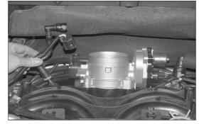
8. Disconnect the TPS sensor electrical connection from the throttle body and then remove the four throttle body mounting bolts.
