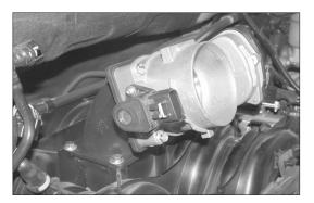
11. Install the throttle body assembly onto the intake manifold with the hardware provided as shown.
