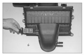
21. Remove the two screws that secure the mass air sensor to the air box with the wrench provided, then remove the mass air sensor.
