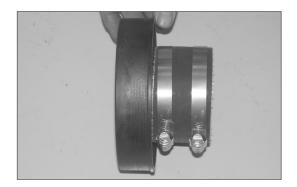
34. Install the silicone hose (#08630) onto the K&N<sup>®</sup> filter adapter and secure with the provided hose clamp as shown.
