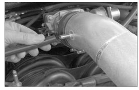
29. Install the provided silicone vent hose onto the valve cover and onto the  $K\&N^{\circledast}$  intake tube as shown.
