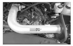
27. Install the K&N<sup>®</sup> intake tube onto the throttle body and position so that it lines up with the tube mounting bracket installed in step #25. Secure the intake tube with the provided bolt and hose clamp.
