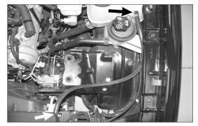
14. Install the supplied coolant recovery hose and secure with the provided hose clamps. NOTE: Be sure to replace the coolant that was recovered during hose removal by replenishing it in the coolant recovery tank.
