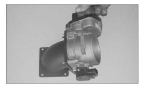
10. Using the bolts removed in step #8, secure the throttle body to the throttle body adapter with the gasket as shown.
