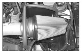
36. Install the K&N<sup>®</sup> air filter assembly onto the K&N<sup>®</sup> intake tube as shown and secure with the provided hose clamp.
