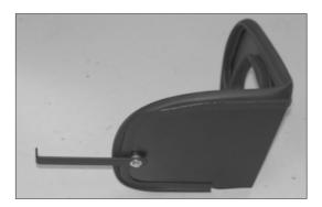
17. Install the "L" bracket (#070026) onto the heat shield with the provided spacer and hardware as shown.
