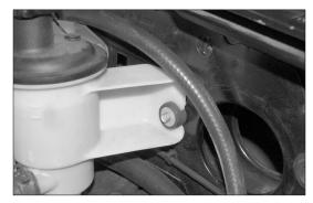
19. Remove the power steering reservoir mounting bolt shown.
