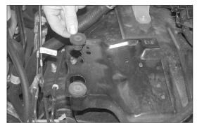
18. Install the provided nut inserts into the air box mounting holes as shown.
