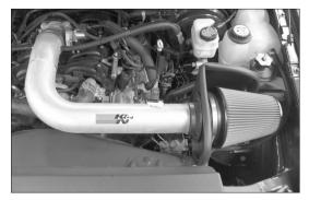
37. Reconnect the vehicle's negative battery cable. Double check to make sure everything is tight and properly positioned before starting the vehicle.
