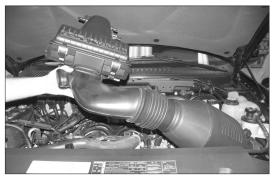
7. Lift the air filter housing and remove the entire intake tube and filter assembly from the inner fender of the vehicle.
