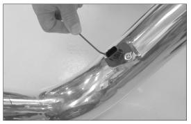
22. Install the mass air sensor into the  $\text{K\&N}^{\otimes}$  intake tube and secure with the provided hardware as shown.
