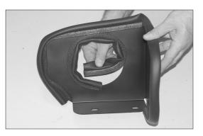
16. Install the short edge trim into the hole in the heat shield as shown.
