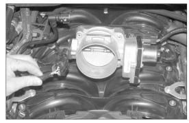
12. Reconnect the throttle body motor and TPS electrical connections.
