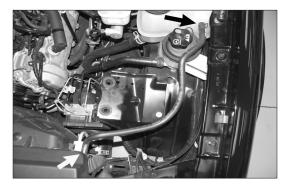
13. Loosen the coolant recovery hose, hose clamps, and then remove the factory recovery hose shown. Be sure to catch any coolant, which flows out of the radiator during hose removal.
