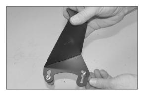
24. Pass the two valve cover bolts removed in step #23 through the keyhole slots in the tube mounting brackets as shown.
