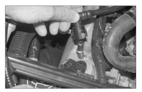
28. Unlock the crank case vent hose and remove the hose from the valve cover.
