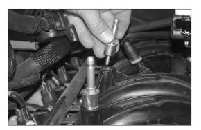
31. Re-install the factory air box mounting studs with the provided spacers as shown.
