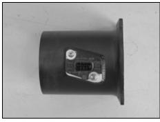
14. On 2006 models, install the mass air sensor removed in step #13 into the mass air sensor housing with the supplied hardware as shown.
