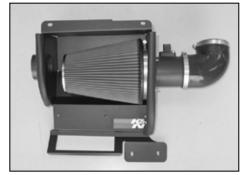
24. Install the K&N<sup>®</sup> air filter onto the filter adapter
