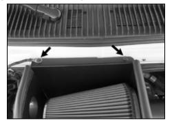
30. Using the factory bolts removed in step #3, secure the heat shield to the cowl. NOTE: Be sure the spacers are in position and to attach the ground strap.
