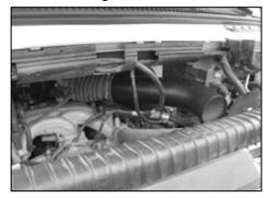
26. Install the K&N<sup>®</sup> intake tube into the bellows at the throttle body and secure with the factory hose clamp.
