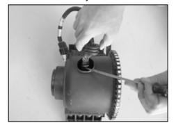
10. Pull back the rubber plug to gain access to the primary mass air sensor connection. Using a small screw driver, release the locking tab and disconnect the mass air sensor electrical connection.
