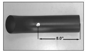
25a. On vehicles equipped with an external temperature sensor; measure and mark the tube 8.0" (from the straight end of the tube, on the inside radius of the bend). Then, drill a 5/8" ID hole in the tube as shown.
