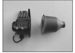
9. Unlatch the clam shell connector and separate the air filter assembly as shown.
