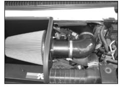
29. Insert the K&N<sup>®</sup> intake tube into the silicone hose at the throttle body and secure with the provided hose clamp.
