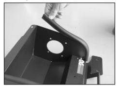
16. Install the long edge trim to the heat shield as shown. Some trimming of the edge trim may be necessary.
