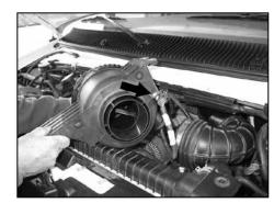
6. Lift up the air filter housing and unhook the mass air sensor secondary connector from the housing. Then disconnect the mass air sensor secondary connection and remove the filter assembly from the vehicle.
