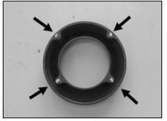
17. Install the four supplied m6 studs into the filter adapter as shown.
