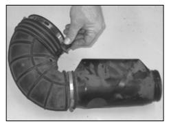
8a. On vehicles equipped with an external air temperature sensor; remove the air temperature sensor from the stock intake tube. **NOTE: The air temperature sensor is fragile; take care when removing.**
