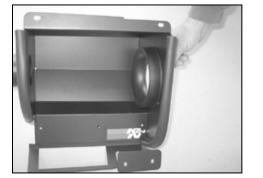
19. Install the filter adapter into the heat shield as shown.
