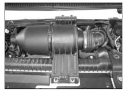
5. Remove the two bolts that secure the air filter housing to the radiator core support. NOTE: These two bolts will be reused. NOTE: Some models may come equipped with a plastic cowl cover that conceals the air box mounting bolts. It will be necessary to remove the cover mounting screws and then remove the cover for access the bolts and modifications to the cover.
