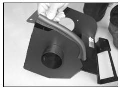
15. Install the short edge trim to the heat shield as shown. Some trimming of the edge trim may be necessary.
