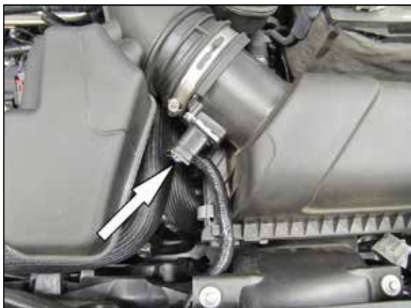
2. Disconnect the mass air sensor electrical connection.
