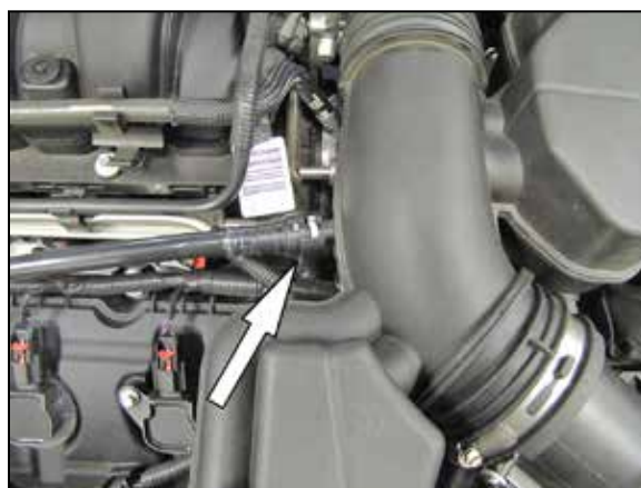
3. Disconnect the crank case vent tube from the factory intake tube.
