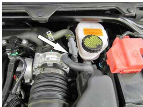
4. Disconnect the EVAP vent line from the check valve as shown.
