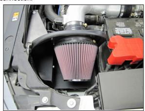
27. Install the  $K\&N^{\otimes}$  air filter and secure with the provided hose clamp.
