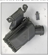
16. Remove the two screws securing the mass air sensor into the factory air box and then remove the mass air sensor from the air box.
