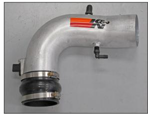
19. Install the silicone hump hose (084057) onto the  $K\&N^{\odot}$  intake tube as shown.
