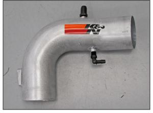
15. Install the 90° vent and the straight vent fitting into the K&N® intake tube as shown.
