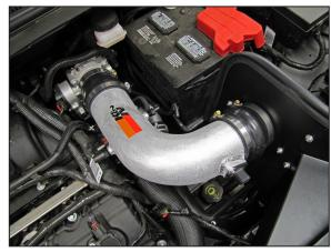
20. Install the K&N® intake tube into the silicone hose at the throttle body then align with the filter adapter, slide the silicone hump hose onto the filter adapter. Secure the intake tube with the provided hose clamps.
