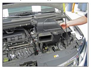
9. Lift up and remove the air box assembly from the vehicle.
