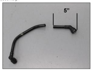
23. Measure 5" from the intake tube end of the crank case vent tube and then cut the crank case vent tube as shown.
