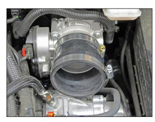
18. Install the silicone hose (08724) onto the throttle body and secure with the provided hose clamp.
