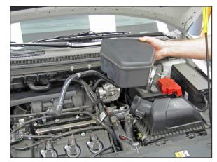
7. Remove the intake tube assembly from the vehicle.
