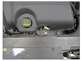
3. Remove the nut securing the front of the engine cover.
