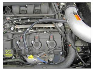
25. Reinstall the crank case vent tube onto the valve cover port and then install the open end to the fitting installed into the K&N® intake tube as shown.
