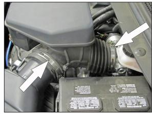
6. Loosen the two hose clamps securing the intake tube assembly to the throttle body and air filter housing.
