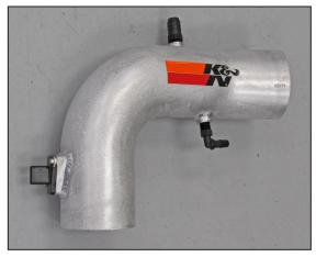
17. Install the mass air sensor into the  $K\&N^{\mbox{\scriptsize @}}$  intake tube and secure with the provide hardware.
