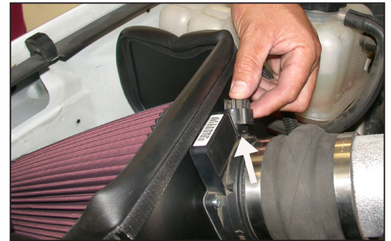
19. Reconnect the mass air sensor electrical connection as shown.
