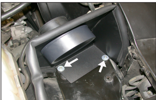
13. Secure the heat shield to the rubber mounted studs using the provided hardware but do not tighten at this time.
