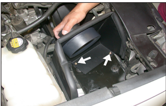
12. Install the heat shield onto the rubber mounted studs as shown.
