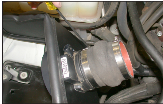
15. Install the silicone step hump hose and hose clamps onto the mass air sensor and tighten as shown.
