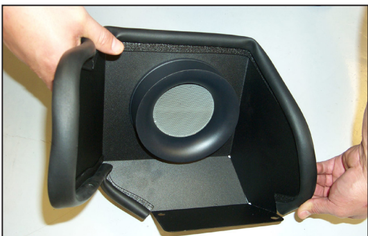
11. Install the edge trim onto the heat shield as shown.
