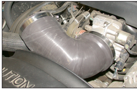
14. Install the silicone angled hose and hose clamps onto the throttle body but do not tighten at this time.
