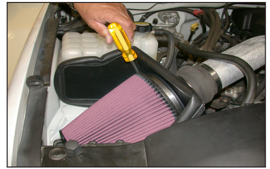
18. Install the K&N® air filter onto the mass air adapter and secure with the provided hose clamp as shown.
