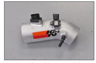
18. Install the 90° vent fitting into the K&N® intake tube as shown.
