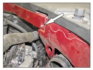
12. Remove the bolt shown in the core support.
