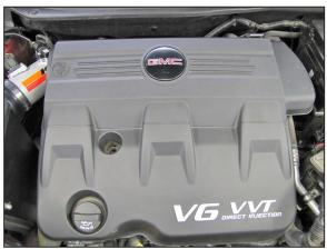
28. Reinstall the engine cover and secure with the factory bolt and oil filler cap.
