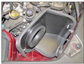
15. Set the heat shield assembly into position and secure with the provided hardware.
