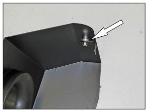
9. Install one of the provided "L" brackets (070066) onto the heat shield as shown using the provided hardware and spacer.
