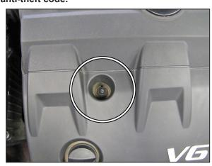
2. Remove the bolt securing the engine cover, remove the oil filler cap and then lift off the engine cover and remove it from the engine. NOTE: reinstall the oil filler cap.
