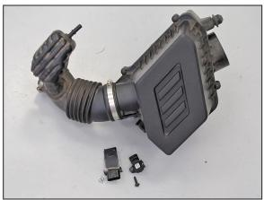
16. Remove the mass air sensor and humidity sensor from the factory air box.
