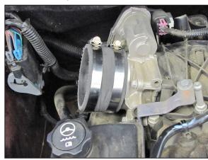
19. Install the provided coupling hose (08186) onto the throttle body and secure with the provided hose clamp.
