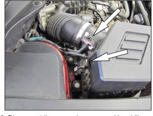
3. Disconnect the mass air sensor and humidity sensor electrical connections.
