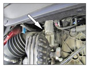
5. Loosen the hose clamp that secures the factory intake tube to the throttle body.
