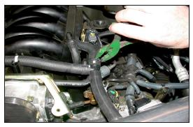
31. Reconnect the crank case vent hoses to the plastic "T" as shown.
