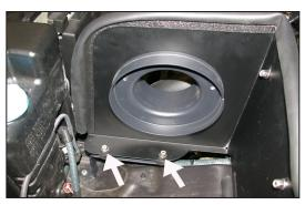
21. Install the heat shield into the vehicle and secure it to the rubber mounted studs using the provided hardware as shown, but do not tighten at this time.
