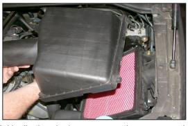
7. Unclip the air cleaner cover, then, remove the air cleaner cover as shown.
