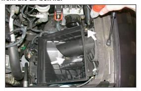
8. Remove the two bolts on the air cleaner as shown.
