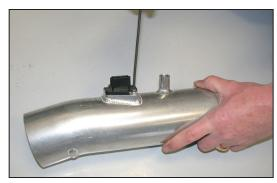
26. Install the mass air sensor into the K&N® intake tube using the provided hardware as shown.
