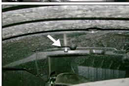
22. Secure the "L" bracket to the hole from step 10 on the inner fender panel with the provided hardware as shown.
