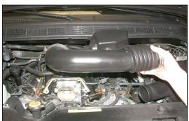
6. Loosen the hose clamps, then, remove the stock intake tube as shown.
