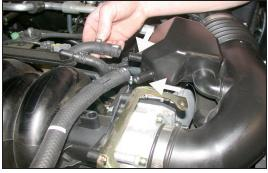
5. Disconnect the crank case vent hoses from the intake tube resonator as shown
