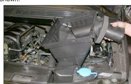
9. Pull firmly upwards to release the air cleaner from the lower grommet as shown.
