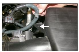
4. Unclip the mass air sensor wire harness from the tab on the air cleaner as shown.
