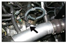
33. Reconnect the mass air sensor electrical connection as shown.
