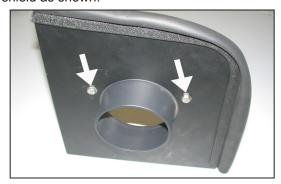
14. Using the provided tube of thread locker, apply two drops to the hex bolts and secure the filter adapter to the heat shield with the provided hex bolts and wave washers as shown.
