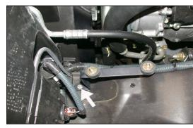
20. Install the "Z" bracket into the vehicle and secure it to the threaded hole from step 11 using the provided hardware as shown.
