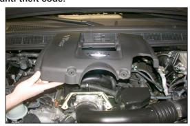
2. Remove the two bolts that secure the engine cover, then, remove the engine cover as shown.
