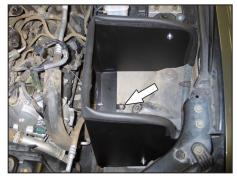
15. Install the heat shield assembly into position and secure with the provided hardware and the bolt removed in the previous step. **NOTE: Be sure to place the ground strap between the heat shield mounting bracket and inner fender.**  tube and secure with the provided hardware.
