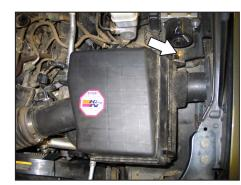
7. Remove the bolt shown which secures the airbox to the inner fender.
