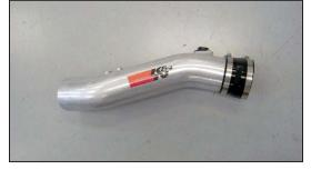
21. Install the provided silicone hose (08051) onto the K&N<sup>®</sup> intake tube as shown and secure with the provided hose clamp.
