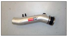
24. Install the two ¼ NPT crankcase vent fittings into the K&N<sup>®</sup> intake tube as shown. **NOTE: Plastic NPT fittings are easy to cross thread. Install the vent fitting "hand" tight, then turn it two complete turns with a wrench.**
