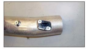
20. Install the mass air sensor into the  $K\&N^{\ensuremath{\circledast}}$  intake
