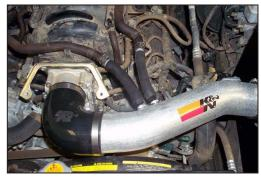
26. Install the K&N<sup>®</sup> intake tube assembly and secure to the mounting bracket and silicone hose with the provided hardware and hose clamp. Then
