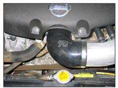
30. Reinstall the engine cover and secure with the factory bolts.
