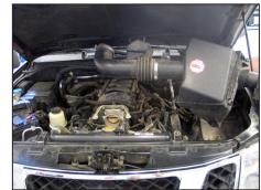
2. Disconnect the mass air sensor electrical connection and unclip the wiring harness from the airbox.
