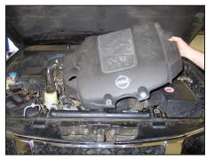
4. Lift the engine cover and dislodge it from the mounting grommets and then remove the engine cover from the engine.
