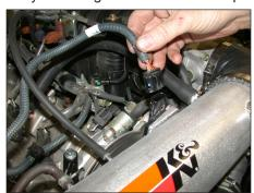
29. Reconnect the mass air sensor electrical connection as shown.
