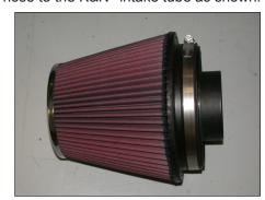
25. Install the filter adapter into the air filter as shown and secure with the provided hose clamp. NOTE: Drycharger® air filter wrap; part number RF-1042DK is available to purchase separately. To learn more about Drycharger® filter wraps or look up color availability please visit http://www.knfilters.com®.
