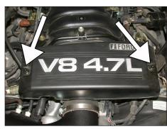
3. Loosen and remove the nuts shown that secure the throttle body cover, then remove the throttle body cover from the engine.
