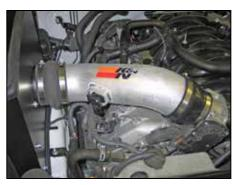
22. Install the K&N® intake tube into the hump hose attached to the heat shield and then into the step hose attached to the throttle body. Secure with the provided hose clamps.
