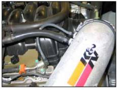
23. Connect the crank case vent hose and the fuel pressure hose to the fittings connected to the K&N<sup>®</sup> intake tube.
