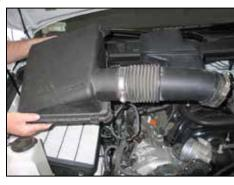
6. Release the four retaining clips securing the upper air box, then remove the upper air box and intake tube assembly from the vehicle.
