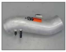
19. Install the provided NPT vent fittings into the K&N® intake tube as shown.
