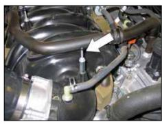
29. Install the mounting stud into the nut extension as shown.
