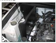
14. Set the heat shield into the engine compartment and secure the factory install nuts with the provided hardware.
