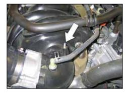
27. Install the provided stud into the mounting stud location as shown.
