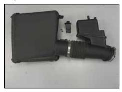
17. Remove the two screws securing the mass air sensor. Remove the mass air sensor from the upper air box housing.
