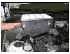
7. Loosen the two bolts securing the lower air box, and then remove the lower air box from the vehicle. NOTE: K&N Engineering, Inc., recommends that customers do not discard factory air intake.
