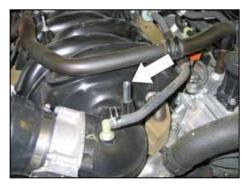
28. Install the provided nut extension onto the stud as shown.
