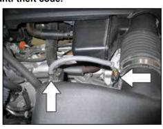
2. Disconnect the mass air sensor electrical connection and then unhook the wiring harness from the air box.
