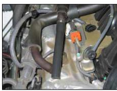
21. Install the crank case vent hose assembly into the factory crank case vent hose as shown.
