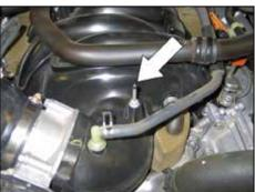
26. Remove the front engine cover mounting stud from the intake manifold.
