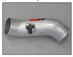
18. Install the mass air sensor into the intake tube and secure with the provided hardware.
