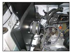
16. Install the silicone hump hose (08418) onto the filter adapter and secure with the provided hose clamp.
