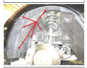
h. Using a flat screw driver, disconnect the six trim panel clips shown above. Disconnect by inserting screwdriver
