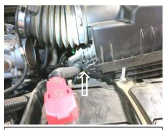
f. Unclip the wiring harness from the stock air box and remove the stock intake system from the vehicle. Note: Do not discard any of your stock equipment.
