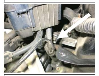
g. Remove the electrical tape that holds the MAF harness to the main wire harness.
