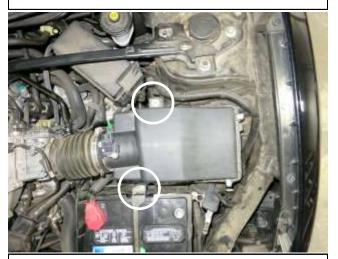
d. Remove the two bolts circled that secure the air box to the vehicle.
