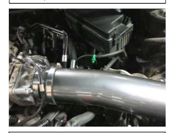
d. Install the AEM intake tube into the coupler that was previously installed. Do not tighten the hose clamp at this time.
