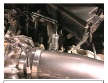
f. Install the provided hose and spring clamp onto the AEM intake tube. Install the vent line into the hose and secure the spring clamp that was removed in step 2c. Note: Trim hose to fit.
