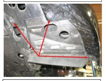
the clip can then be pulled out together. Repeat for the three clips in front of the wheel shown above.
