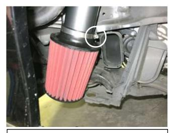
i. Install the AEM filter onto the AEM tube and secure with the provided hose clamp to 30 in-lbs.
