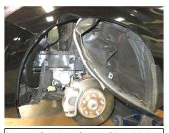
k. Once the fender liner is free, it can fold neatly back behind the brake assembly as shown.
