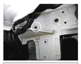
a. Install the provided wellnut into the frame of the vehicle as shown. Note: Use soap and water to ease installation.
