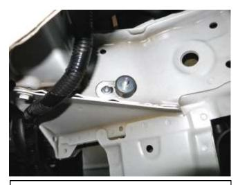
e. Install the rubber mount onto the provided bracket & install the bracket into the vehicle, then secure the screw to the wellnut. Align the AEM intake tube bracket with the mount & secure with provided washer & nut.
