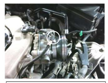
b. Install the included coupler and hose clamps as shown on the throttle body. Tighten the one closest to the throttle body to 30 in-lbs.
