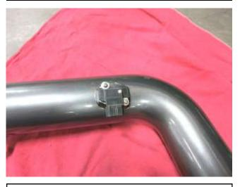
c. Install the MAF sensor with factory screws removed in step 2m onto the AEM intake tube.
