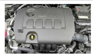
3. Lift up the decorative engine cover to release it from the mounting grommets and then remove from the vehicle.
