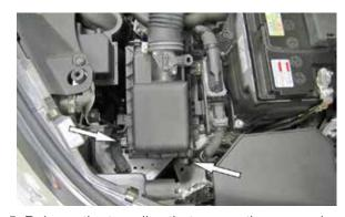
5. Release the two clips that secure the upper air filter housing, then remove the upper housing with the intake tube and crank case breather hose. Remove the factory air filter.
