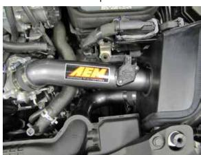
16. Install the AEM® intake tube through the heat shield and then into the coupler at the throttle body, adjust the tube for best fit and then secure with the provided hose clamp.
