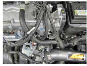
18. Install the provided crank case vent hose onto the fitting on the intake tube and then onto the fitting on the valve cover.
