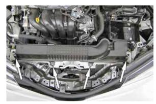
7. Remove the four bolts that secure the fresh air inlet duct and then remove the duct from the vehicle.
