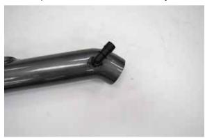
14. Install the provided 90° vent fitting into the intake tube as shown.
