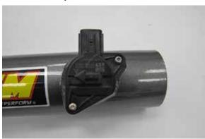
15. Remove the mass air sensor from the factory air filter housing and install it into the AEM® intake tube and secure with the provided hardware.
