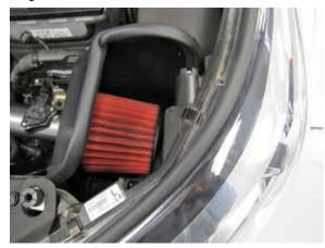
19. Install the AEM® air filter and secure with the provided hose clamp.
