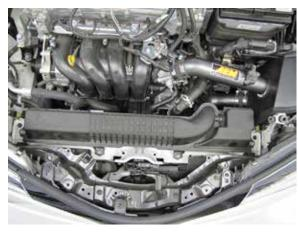
17. Install the factory fresh air intake and align the AEM® fresh air intake tube. Secure the factory fresh air intake with the factory bolts and secure the AEM® fresh air tube with the hose clamp provided.
