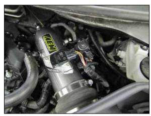
25. Reconnect the mass air sensor and EVAP solenoid electrical connections. Connect the EVAP vent line if equipped.
