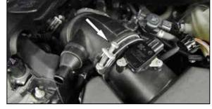
5. Loosen the hose clamp that secures the factory intake hose to the air filter housing.
