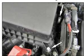
6. Release the two clips that secure the upper air filter housing, remove the upper air filter housing and factory air filter.
