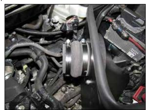
21. Install the provided hump coupler (084079) onto the filter adapter installed into the heat shield and secure with the provided hose clamp.
