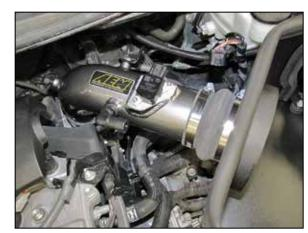
22. Install the AEM® intake tube into the coupler hoses, align for best fit and then secure with the provided hose clamps.
