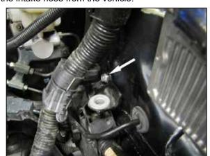
10. Remove the bolt that secures the rear air filter housing mounting bracket to the strut tower and remove the bracket from the vehicle.
