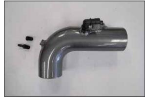
19. Install the EVAP vent fitting into the AEM® intake tube. On vehicles that are not equipped with the EVAP vent hose from the factory install the npt plug into the AEM® intake tube.
