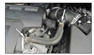
4. Release the spring clamps and remove the crank case vent line from the valve cover and intake tube.
