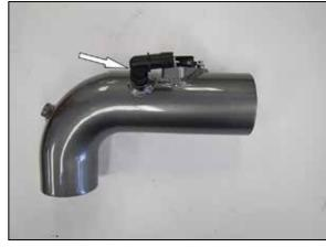
18. Install the  $90^{\circ}$  vent fitting into the AEM® intake tube as shown.
