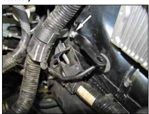
14. Install the heat shield mounting bracket (070702) onto the strut tower air filter housing mounting bracket location from step #10 using the hardware provided.
