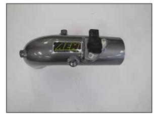
17. Remove the mass air sensor from the factory air filter housing and install it into the AEM® intake tube using the provided hardware.
