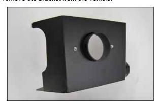
11. Install the filter adapter into the heat shield and secure with the provided hardware.
