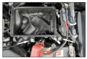
7. Remove the two bolts that secure the lower air filter housing. Lift up the lower air filter housing to unhook it from the mounting grommet and disconnect it from the fresh air duct. Then remove the lower housing from the vehicle.
