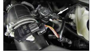
3. Disconnect the EVAP solenoid electrical connection.
