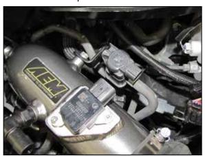
23. Secure the EVAP solenoid to the bracket installed onto the intake tube using the factory screw.
