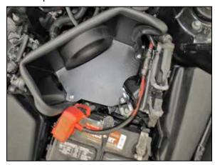
15. Install the heat shield into the vehicle so the fresh air duct slides over the fresh air tube on the heat shield. Secure the heat shield with the hardware provided.
