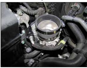
16. Install the provided coupler hose (5-302) into the throttle body and secure with the provided hose clamp.
