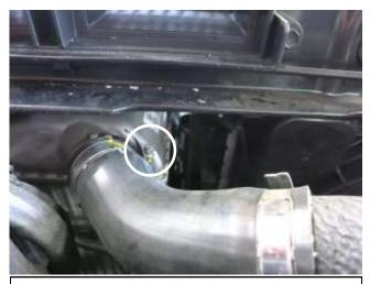
g. Loosen the hose clamp at the intercooler. Note: A hose clamp cap that covers the slot may be present. You can pry it off with a screwdriver or pliers.
