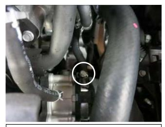
i. Loosen the hose clamp at the throttle body.
