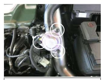
n. Reinstall the BOV onto the AEM intercooler pipe and tighten with the bolts that were removed in step 2d.
