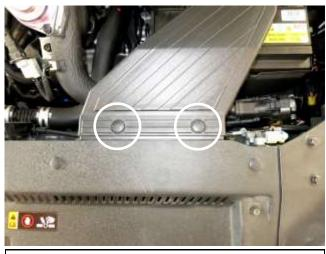
a. Remove the two clips securing the stock air scoop to the vehicle.
