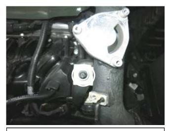
e. Remove the bolt that secures the intercooler pipe to the engine. This bolt will not be reused.
