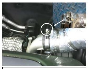
f. Loosen the hose clamp at the turbo compressor. Note: A hose clamp cap that covers the slot may be present. You can pry it off with a screwdriver or pliers.
