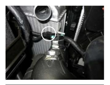
f. Connect the pressure sensor electrical connecter to the pressure sensor.
