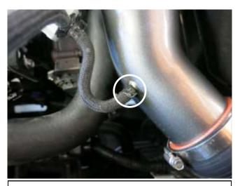
m. Reattach the vacuum hose that was removed in step2c. with the stock spring clamp.
