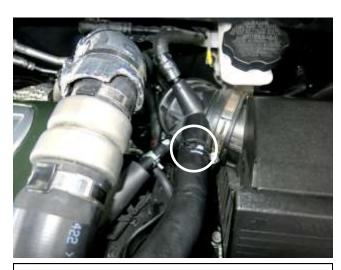
b. Squeeze the spring clamp and work the clamp back off of the turbo recirculation valve hose. Disconnect the hose from the stock intake arm.
