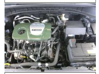
h. Remove the upper intercooler pipe from the engine.
