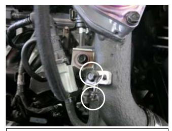
c. Remove the M6 bolt securing the electrical connector. Squeeze on the spring clamp and remove the vacuum hose from the nipple. These will be reused in step 3l & 3m.
