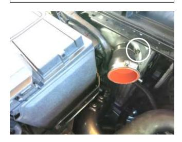
h. Install the provided coupler and hose clamps onto the intercooler. Tighten the hose clamp circled at this time to 30 in-lbs.
