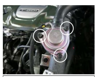
d. Remove the 3 bolts securing the recirculation valve to the stock intercooler pipe, then move the valve to the side of the engine compartment. Note: Do not lose the O-ring under the valve.
