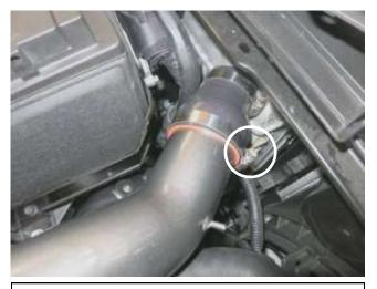
$\ensuremath{k}.$  Tighten hose clamp circled at the intercooler to 30 inlbs
