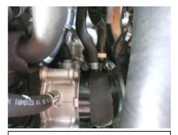
e. After installing the coupler and hose clamps onto the throttle body, make sure the tube is aligned and tighten the all the hose clamps at the throttle body and lower intercooler outlet to 30 in-lbs.
