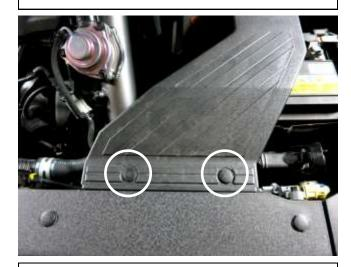
p. Install the stock scoop back into the vehicle with the clips removed in step 2a.
