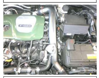
i. Install the AEM upper intercooler pipe into the previously installed couplers. Note: Using warm soapy water may help installation and alignment.
