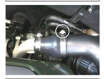
j. Once the AEM intercooler pipe is properly aligned. Tighten the hose clamp circled to 30 in-lbs.
