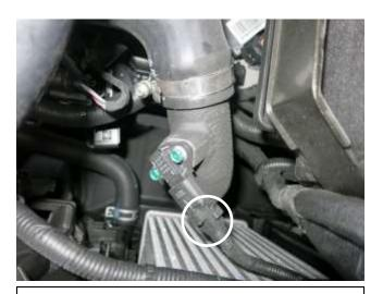
j. Remove the electrical connector from the pressure sensor on the lower intercooler pipe.
