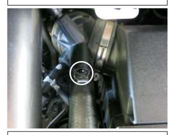
o. Slide the BOV hose back onto the stock intake tube and secure with the stock spring clamp that was removed in step 2b. Note: Soapy water will help with installation.
