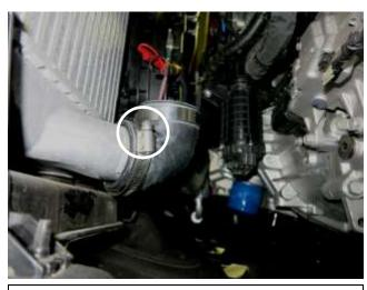
b. Install the 90° coupler with the provided hose clamps onto the lower intercooler outlet. Note: Warm soapy water will help with installation.
