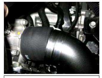
d. Install the provided coupler into the throttle body and install the AEM lower intercooler pipe into the coupler along with hose clamps. Note: Warm soapy water will help with installation.
