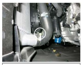
I. Loosen the hose clamp at the lower intercooler outlet from under the vehicle. Note: A hose clamp cap that covers the slot may be present. You can pry it off with a screwdriver or pliers.
