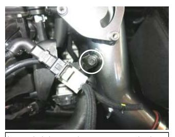
I. Using the bolt removed in step 2c to secure the electrical connector to the AEM pipe.
