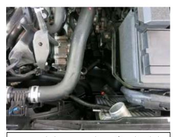
$\ensuremath{\mathsf{m}}.$  Remove the lower intercooler pipe from the vehicle.
