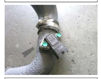
n. Remove the two M6 bolts securing the pressure sensor to the lower intercooler pipe. These bolts will not be reused.
