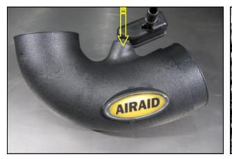
**10.** Transfer the PCV fitting into the Intake tube and apply the Airaid Decal as shown.
