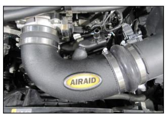
12. Insert the Intake Tube into the coupler first, then into the Hump Hose. Tighten all four clamps at this time.
