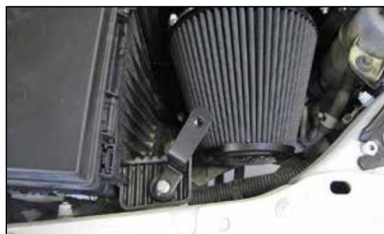
17. Install the provided bracket (083163) onto the rubber mounted stud using the provided hardware.
