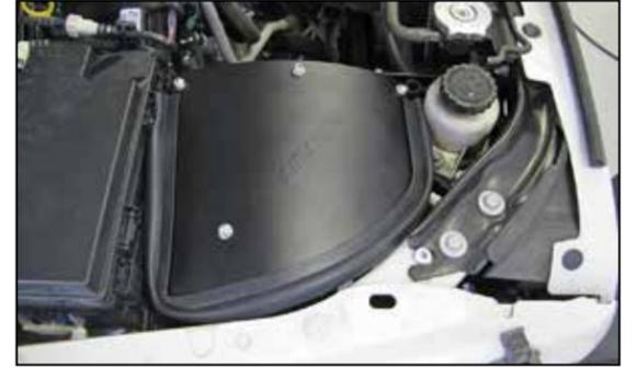
18. Install the AIRAID filter lid and secure with the provided hardware.
