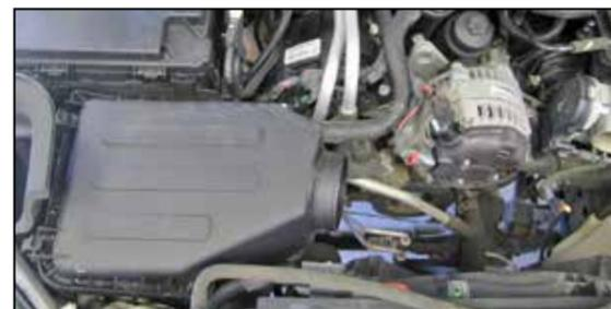
5. Disconnect the crank case vent hose from the crank case vent tube. Lift up and remove the air filter housing from the vehicle.
