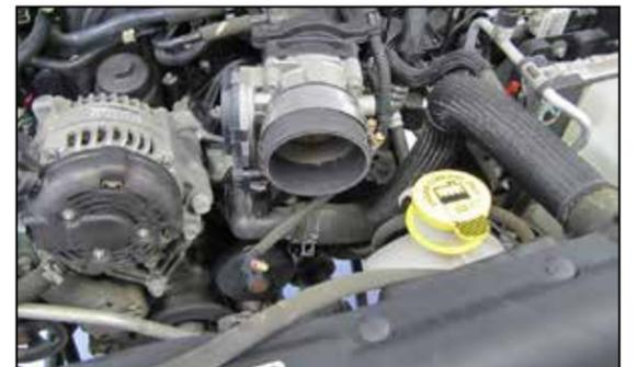
20. Install the provided silicone hose (08690) onto the throttle body and secure with the provided hose clamp.
