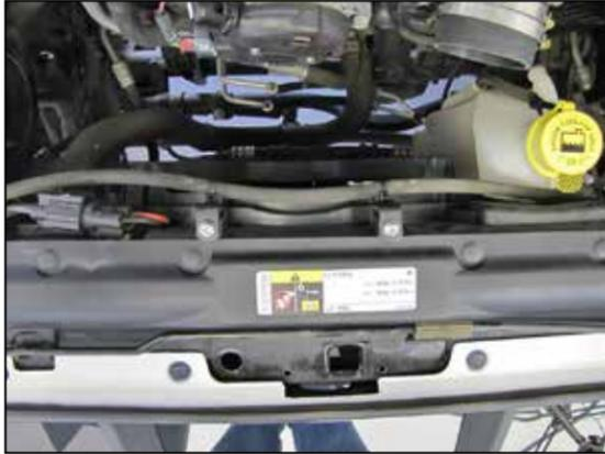
25. Install the tie wrap equipped brackets onto the factory intake tube mounting locations on the fan shroud using the provided hardware. Then secure the coolant over flow hose with the tie wraps.
