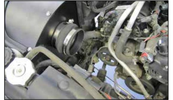
19. Install the provided hump hose (08699) onto the filter adapter and secure with the provided hose clamp.
