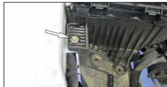
6. Remove the bolt shown that secures the air box mount bracket to the inner fender.
