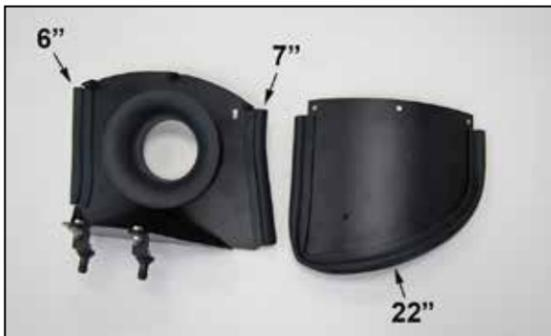
11. Cut the provided edge trim into three sections. One section is to be 6" long, one section is to be 7" long and the final section is to be 22" long. Install the edge trim onto the heat shield and lid as shown.
