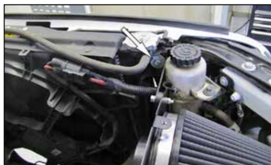
15. Install the heat shield bracket assembly onto the heat shield and radiator mount as shown. Secure the bracket with the factory bolt from step number 7 and the hardware provided.
