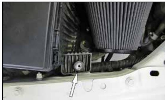
16. Install the rubber mounted stud into the air box mounting plate bolt location as shown.
