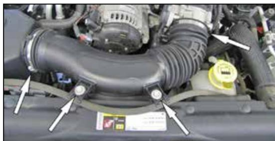
3. Remove the two bolts which secure the factory intake tube to the fan shroud. Loosen the hose clamp securing the factory intake tube to the air filter housing. Loosen the hose clamp securing the factory intake tube to the throttle body.
