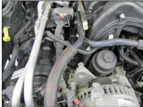
28. Connect the open end of the crank case vent hose to the factory crank case vent tube as shown.
