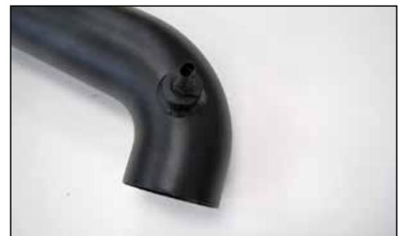
23. Remove the inlet air temperature sensor from the factory intake plenum then install the inlet air temperature sensor into the AIRAID intake tube as shown.
