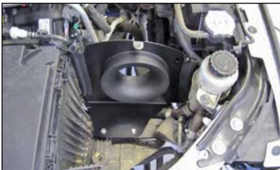
12. Install the heat shield assembly into position so the mounting studs are in the air box mounting grommets.
