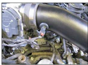
20. Reconnect the inlet air temperature sensor electrical connection.
