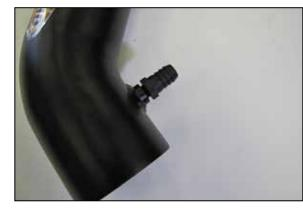
17. Install the provided vent fitting into the AIRAID® intake tube as shown.
