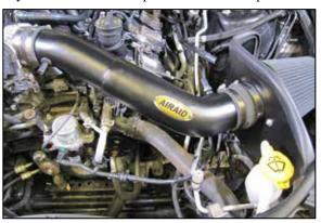
19. Install the AIRAID® intake tube into the coupler at the throttle body and then into the hump coupler, adjust the tube for best fit and then secure with the provided hose clamps.
