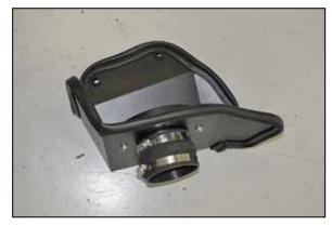
12. Install the provided hump coupler (08699) onto the filter adapter and secure with the provided hose clamp.
