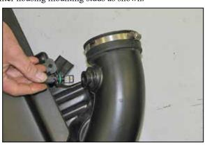
15. Remove the inlet air temperature sensor from the factory intake tube.
