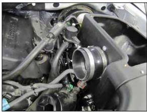
16. Install the coupler hose onto the filter adapter and secure with the provided hose clamp.
