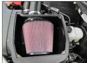
23. Install the AIRAID air filter onto the adapter and secure with the provided hose clamp.
