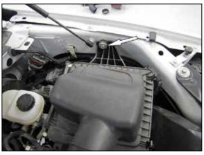
5. Remove the bolt which secures the factory air filter housing to the inner fender. Remove the factory air filter housing and fresh air intake from the vehicle.
