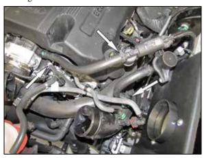
15. Install the modified crank hoses onto the solenoid valves and turbo intake tubes.
