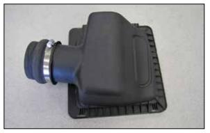
7. Install the provided hump coupler (08639) onto the air filter housing and secure with the provided hose clamp.
