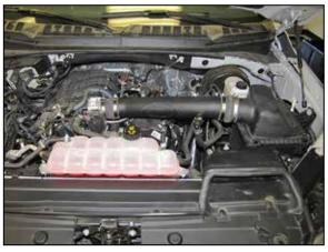
12. Double check your work! Make sure there is no foreign material in the intake path. Make sure all clamps, hoses, bolts, and screws are tight. Double check the hood clearance! **Reconnect the negative battery cable!**
