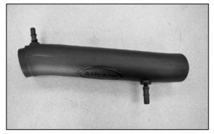
8. Install the two provided quick disconnect vent fittings into the AIRAID® intake tube as shown.
