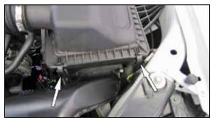
5. Release the clips that secure the upper air filter housing and then remove the upper housing and factory intake tube.
