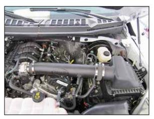
10. Assemble the AIRAID® intake tube and upper air filter housing together loosely, then install the system onto the throttle body and lower housing. Latch the upper air filter housing into position and adjust the intake tube for best fit, then secure with the provided hose clamps.
