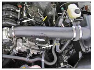
11. Connect the two vent lines to the quick disconnect fittings installed into the intake tube and secure the EVAP line to the insert on the bottom side of the tube.
