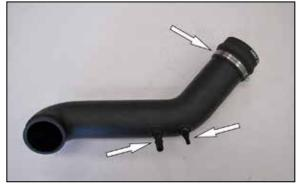
6. Install the provided vent fittings into the AIRAID® intake tube as shown. Install the provided hump coupler (08683) onto the intake tube and secure with the provided hose clamp.
