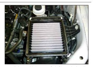
5. Install the provided AIRAID $^{\text{@}}$  air filter and reinstall the factory upper air filter housing.
