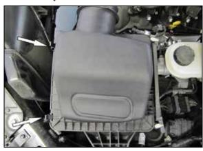
4. Release the two clips that secure the upper air filter housing and then remove the upper housing and factory air filter.
