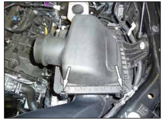
5. Release the two clips securing the upper air filter housing and then remove the upper filter housing and stock air filter.
