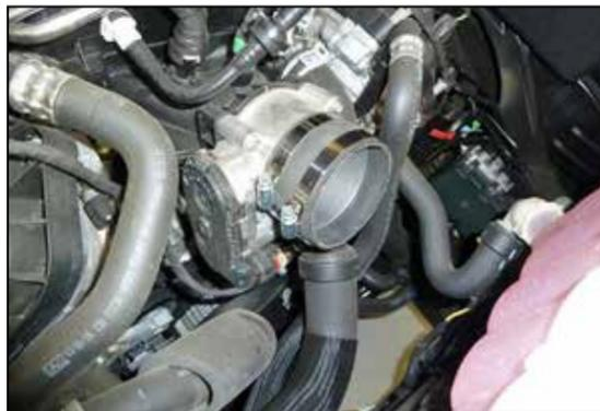
13. Install the provided coupling hose onto the throttle body and secure with the provided hose clamp.
