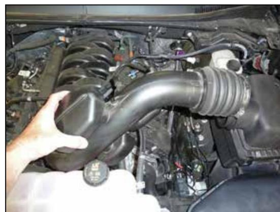
4. Unhook the coolant line from the intake tube and then remove the intake tube from the vehicle.
