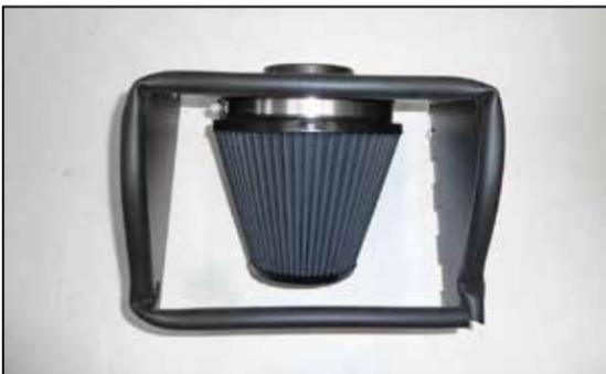
10. Install the air filter onto the filter adapter and secure with the provided hose clamp.
