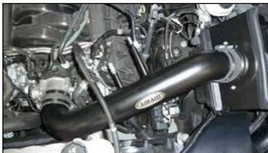
14. Install the AIRAID® intake into the coupling hose at the filter adapter and then into the hose at the throttle body, adjust the tube for best fit and then secure with the provided hose clamps.
