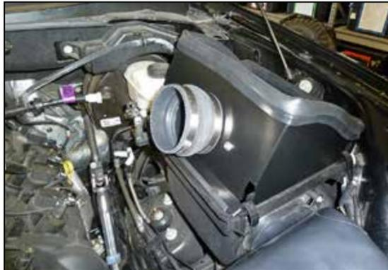
12. Install the provided coupling hump hose onto the filter adapter and secure with the provided hose clamp.
