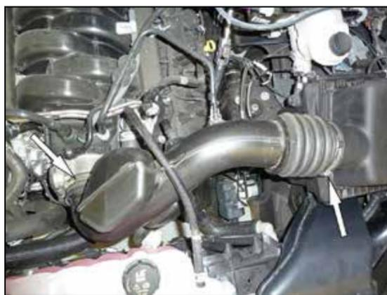
3. Loosen the hose clamps at the throttle body and filter inlet that secure the factory intake tube.
