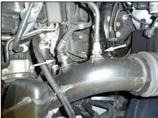
2. Disconnect the EVAP vent connection and crank case vent connection.
