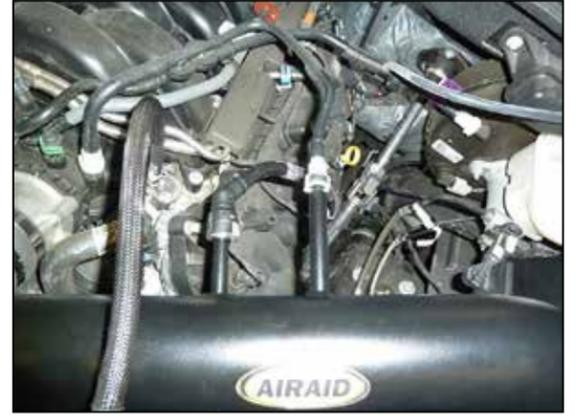
15. Connect the factory EVAP and Crank case vent lines to the fittings on the AIRAID® intake tube.
