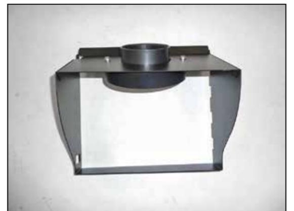
6. Install the filter adapter into the AIRAID® heat shield and secure with provided hardware.
