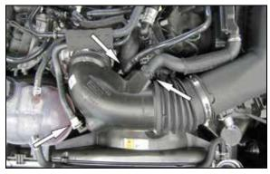
4. Release the spring clamp that secures the sound tube to the intake tube fitting and then disconnect the sound tube from the intake tube. Disconnect the quick connect vent lines shown.
