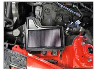
8. Release the clips the secure the upper air filter housing and then remove the factory air filter. Install the AIRAID® replacement air filter and resecure the upper housing with the factory clips.
