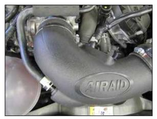
12. Install the AIRAID® intake tube assembly into the coupler hoses, adjust for best fit and then secure with the provided hose clamps. Connect the factory vent lines to the fittings installed into the intake tube.
