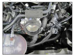
9. Install the provided coupler onto the throttle body and secure with the provided hose clamp.
