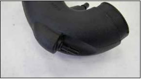
11. Install the provided vent fittings into the AIRAID® intake tube as shown.
