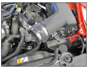
10. Install the provided coupler hose onto the air filter housing and secure with the provided hardware.
