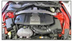
14. Double check your work! Make sure there is no foreign material in the intake path. Make sure all clamps, hoses, bolts, and screws are tight. Double check the hood clearance! Reconnect the negative battery cable!
