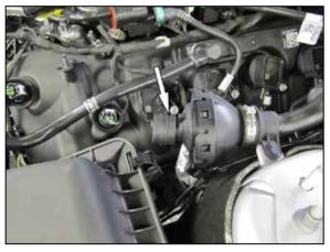
7. Install the provided caplug onto the sound drum.
