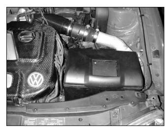
AEM® intake system installed
