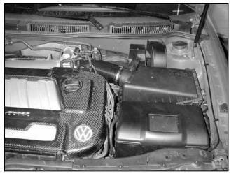
Factory air box system installed
