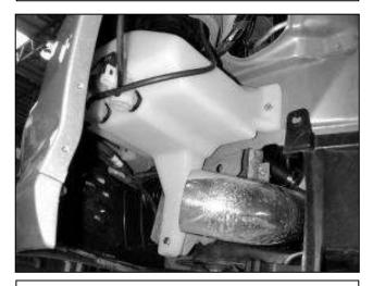
f. Secure the new washer bottle with the three air box bracket bolts removed in step 3c. Reconnect the two feeder lines and the two electrical connectors to the pumps.
