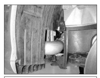
r. Install the left fender well lining and lower splashguard that were removed in step 1eii. The fender liner must be trimmed for the intake system to fit properly. Trim and reinstall the fender liner as shown. Failure to do so will void the warranty.
