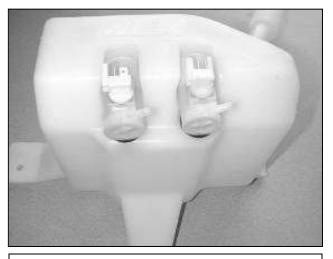
e. Reinstall the two pump grommets and the fill tube grommet on the replacement washer bottle as shown. Wet the grommets with soapy water and insert the two washer pumps and fill tube.
