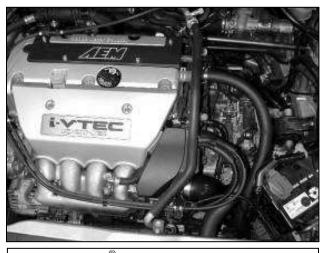
AEM® intake system installed
