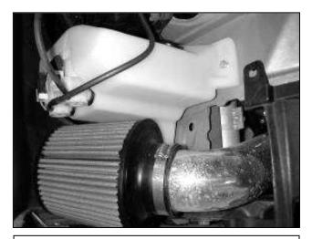
k. Install the  $\mathsf{AEM}^{^{\tiny\textcircled{\tiny{\$}}}}$  air filter onto the lower end of the intake pipe.
