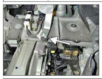
g. Loosely secure the mounting bracket with the remaining fender washer and lock nut. Refer to the diagram below for proper rubber mount installation.
