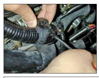
p. Place a small screwdriver in the slot of the clip and gently pry downwards. Split the housing of the clip open. Slide the clip down the wire harness a couple of convolutions to free up more harness towards the MAF sensor. Repeat for the second wire harness clip. Reinstall both clips to the bracket on the engine. Plug in the MAF sensor wire harness and make sure the wires are not stretched.
