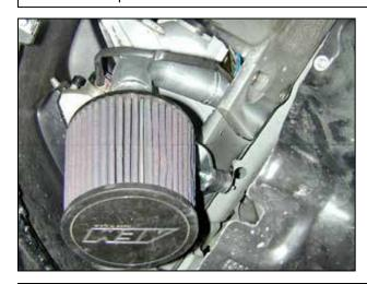
h. Install the AEM® air filter onto the end of the intake pipe.
