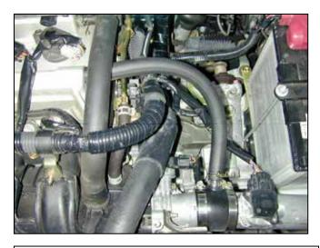
m. Install the supplied breather hose between the nipple on the throttle body coupler and the valve cover. Secure the hose with the original spring clamps.
