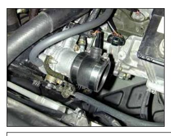
e. Loosely install the coupler onto the throttle body using the two #36 hose clamps. Orient the nipple so that it is pointed approximately 45° back towards the firewall. This will be adjusted later in the installation.
