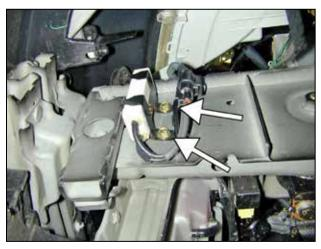
c. Remove the two bolts securing the resistor ballast beneath the driver's side headlight.
