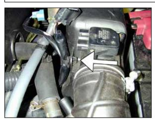
c. Release the wire harness from the air cleaner cover by squeezing the plastic clip from the top and bottom. Carefully remove the plastic clip to allow the MAF and VSV connector harnesses to be routed separately. Remove the breather hose from the vehicle by squeezing the spring clamps on both the intake tube and at the valve cover. Save the spring clamps for use later in the installation.
