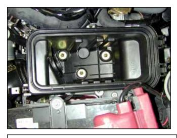
f. Loosen the three bolts that retain the lower air cleaner housing in the engine bay.
