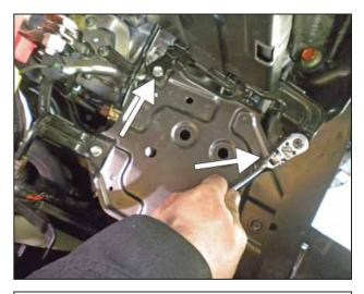
d. Remove two 10mm bolts securing the ECU bracket.
