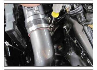
m. Ensure there is sufficient clearance around the intake tubes. Once proper fitment is achieved, tighten all hose clamps and hardware.
