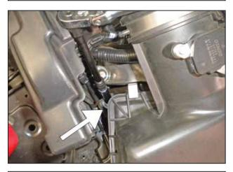
m. Remove the 10mm bolt located at the bottom of the air box.
