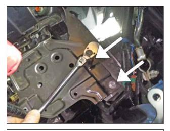
w. Remove the two 12mm bolts on the top of the battery tray.
