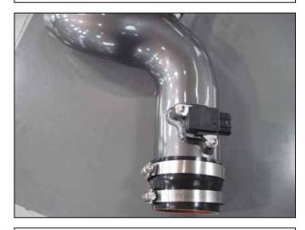
g. Install the reducer coupler on the MAF side of the intake tube.
