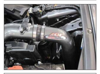
j. Install the lower intake tube as shown.
