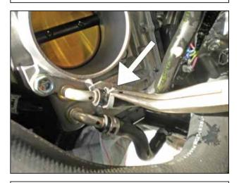
z. CAUTION: Ensure the engine is completely cool before removing the coolant hose, or hot coolant will escape from the cooling system and cause injury or damage. Be sure to capture any lost coolant in a clean container. Release the spring clamp on the throttle body coolant line.
