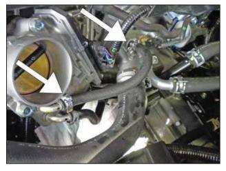
b. Install the supplied 5/16" hose connecting one end to the throttle body hard line and the other to the thermostat housing. Secure the hose with the two supplied small hose clamps.
