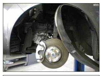
p. Remove the clips securing the fender liner and partially remove the fender liner as shown.
