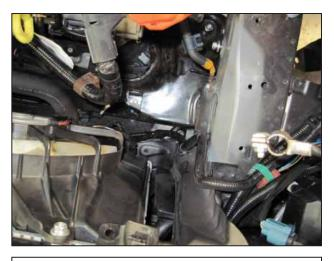
x. Remove the battery tray and intake duct.
