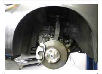
o. Raise the front of the vehicle with a jack. Refer to your owner's manual for proper jack and jack stand placement to properly support vehicle. Support your vehicle using properly rated jack stands before wheel removal or while working under the vehicle. **NEVER WORK UNDER A VEHICLE WITHOUT USING JACK STANDS.** Remove the driver side front wheel.
