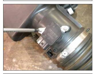
y. Remove the two phillips screws and remove the mass air sensor from the air box assembly.
