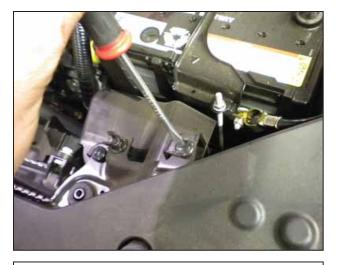
e. Using a flat screwdriver, loosen and remove the two plastic clips securing the resonator bracket. Remove the bracket from the vehicle.
