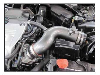
h. Attach the intake tube to the reducer coupler and loosely secure with a #52 hose clamp. Connect the PCV hose to the valve cover. Ensure that the installed intake components are not completely tightened until the installation of the intake system is complete.
