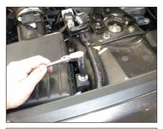
I. Loosen and remove the 10mm bolt at the top of the air box.
