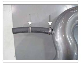
e. Install the supplied 5/8" PCV hose and secure to the intake pipe with the hose clamps as shown.
