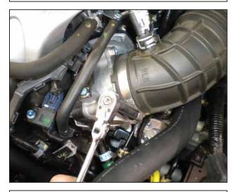
i. Loosen the 10mm hose clamp on throttle body.
