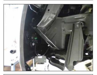
t. The resonator can now be removed from the fender well.
