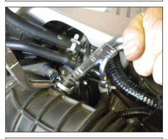
j. Release the spring clamp and remove the PCV hose from the inlet tube.
