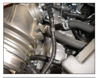
h. Remove the MAF sensor wire from the inlet tube.
