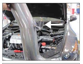
i. Attach the supplied rubber mount onto the lower intake tube bracket as shown.
