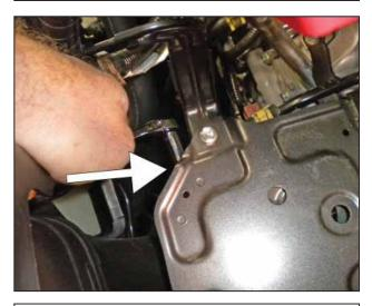
v. Remove the 10mm bolt securing the intake duct.
