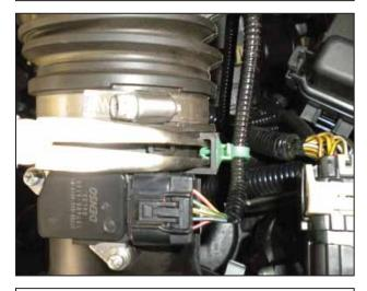
g. Release the zip tie clip that secures the MAF sensor wire to the air inlet assembly.
