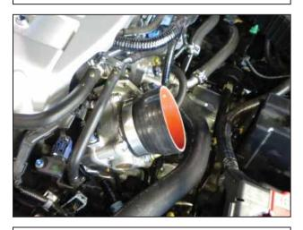
f. Install the reducer coupler on the throttle body.
