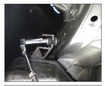
r. Loosen and remove the upper 10mm bolt securing the resonator.
