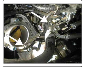
aa. Disconnect the hose clamp at the thermostat housing and remove the coolant and PCV hoses.
