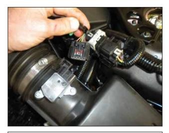
f. Disconnect the MAF sensor wire connector from the MAF sensor.
