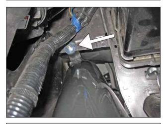
k. Secure the rubber mount previously installed on the intake tube bracket with the provided M6 washer and nut as shown.
