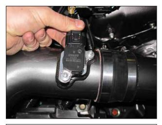
n. Plug in the MAF sensor wire connector into the MAF sensor.
