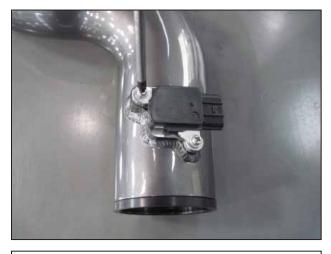
d. Install the MAF sensor using the stock screws.
