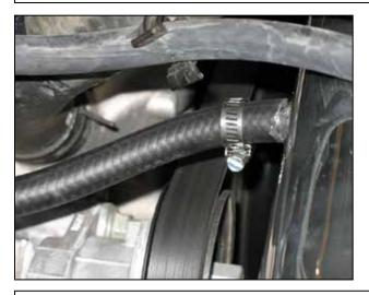
o. Finally, secure the breather hose to the nipple on the intake pipe.
