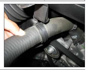
d. Pull the plastic radiator hose tree mount out of the stock intake tube holder.
