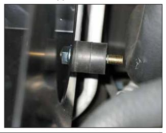
d. Install rubber mount on the heat shield using the supplied washer and nut.
