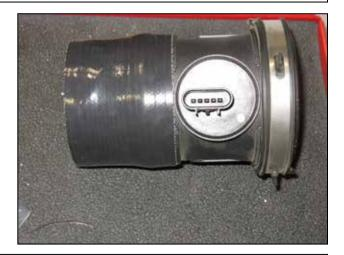
f. Install the reinforced silicone coupler on the MAF housing. Do not put the hose clamps on before attempting to do this.
