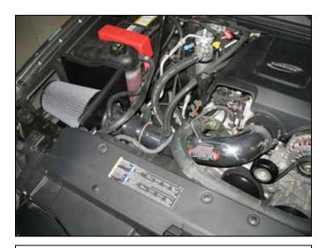
AEM® intake system installed
