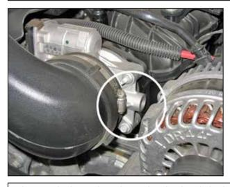
c. Loosen the hose clamp located at the throttle body.
