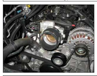
e. Install the reducing coupler on the throttle body, and loosely put the supplied hose clamps on the two ends of the coupler.
