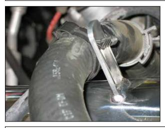
i. Use the stock plastic radiator clamp to secure the radiator hose away from the intake pipe. By inserting it into the bracket located on the pipe.
