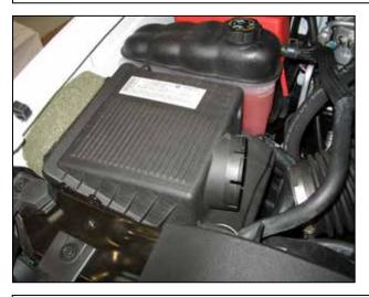
g. Pull the stock air filter housing straight up out of the vehicle.
