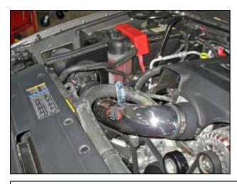
m. Install filter assembly into the stock MAF rubber coupler. Also put the rubber edge gasket along the top edge of the heat shield.
