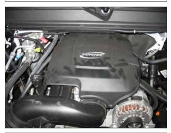
Factory airbox system installed
