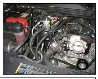
f. Pull the stock inlet tube out of the vehicle.
