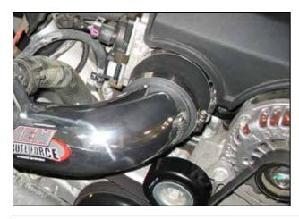
g. Insert intake pipe into reducing coupler located at the throttle body. Route the intake pipe under the upper radiator hose. Secure the bracket to the rubber mount on the heat shield.
