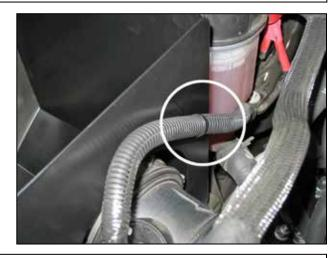
j. Use the supplied tree mount to secure the MAF sensor wire to heat sheild.
