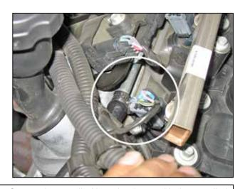
n. Secure the supplied breather hose with the supplied hose clamp.
