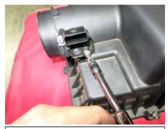
h. Use a T20 Torx bit to remove the MAF sensor from the airbox lid.
