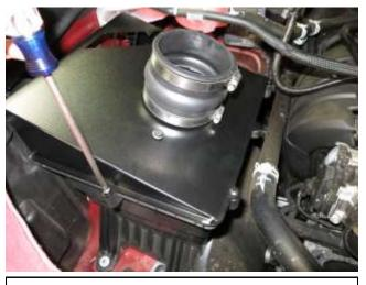
f. Fasten the heat shield to the stock lower airbox using the 4 screws(AEM-1-1020) provided.
