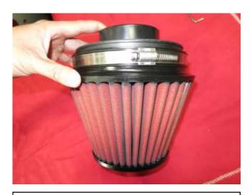
c. Insert the filter adapter(21512-1) into the filter(AEM-21-209D)and fasten with the hose clamp(AEM-94104) provided.
