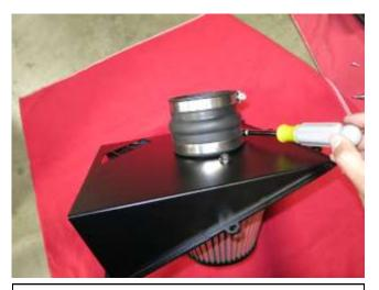
e. Install the hump hose(08657) and fasten it to the adapter using the hose clamp(AEM-9456). Slide hose clamp(AEM-9452) onto the other end.
