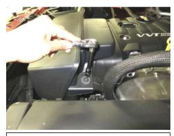
b. Use a T30 Torx bit to remove the indicated bolt on the upper intake resonator.
