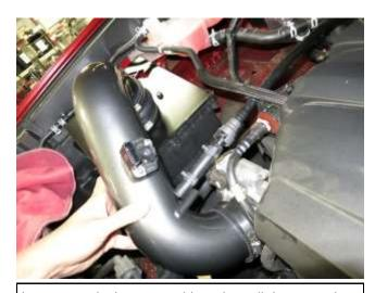
h. Connect the hose assembly and install the AEM tube as shown.
