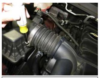
d. Loosen the hose clamp securing the bellow coupler to the airbox lid.
