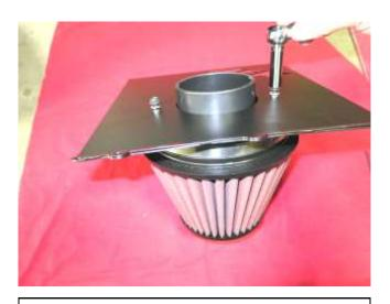
d. Fasten the adapter to the heat shield(AEM-20-8552) using the crush washers(AEM-1-3025) and m6 bolts (AEM-1-2110) provided.
