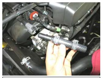
g. Assemble the hose(087028) with the spring clamps (08553) and quick disconnect nipple(082628) provided.
