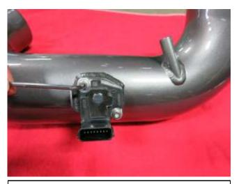
a. Use the provided bolts(07733) to install the MAF sensor into the AEM tube(AEM-2-1533C).
