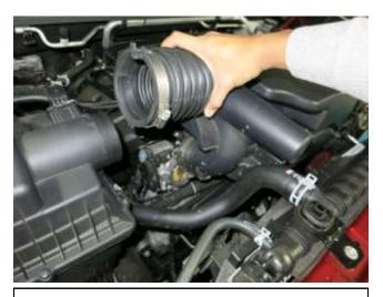
f. Slide the couplers off the airbox lid and throttle to remove the upper resonator assembly.
