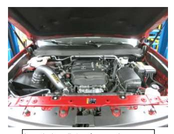
I. Finished installation of AEM Intake System.
