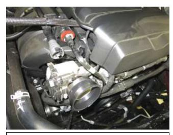
b. Install the coupler(084034) and hose clamps(AEM-9444 and AEM-9452) onto the throttle.
