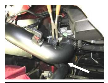
i. Use pliers to slide the spring clamp over the welded nipple. Reconnect the MAF harness to the sensor. Check for clearance with coolant hose and tighten hose clamps.
