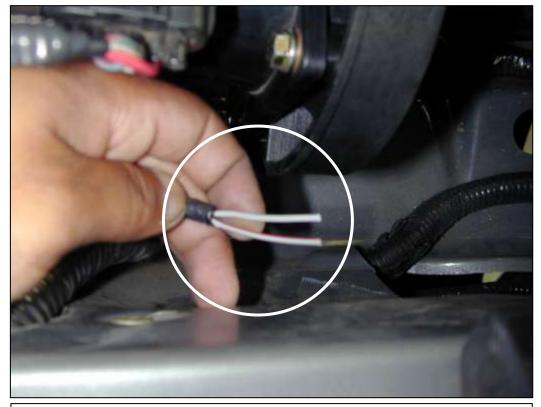
o. Cut back about 2" of wire loom on the remaining IAT harness. Be careful not to cut the wires.
