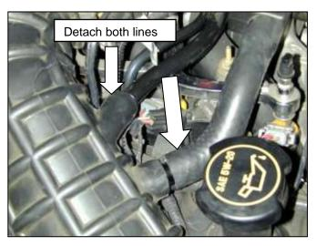
b. Detach the IAC line and the PCV line from the inlet air tube.
