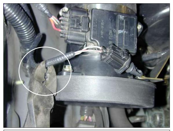
k. Locate the IAT sensor harness. Cut 3" down from the sensor to allow enough wire for crimping.
