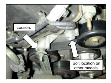
h. Loosen bolt but do not remove. NOTE: On models without individual coils loosen and remove bolt.
