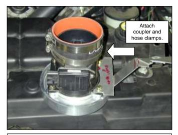
g. Attach coupler and hose clamps. Do not completely tighten.
