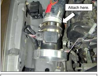
j. Attach the coupler to the inlet pipe. Plug in the MAF sensor harness.
