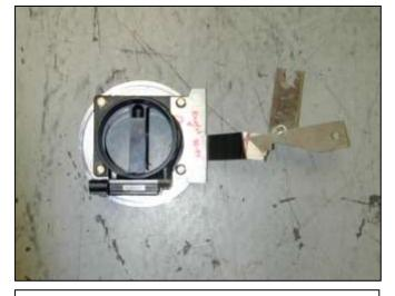
f. Assemble Air horn/MAF sensor adapter to bracket and MAF sensor as shown. Install the provided gasket between the MAF sensor and AEM air horn. The bracket will be on the opposite side of the MAF sensor wiring harness plug. The bracket should point in the same direction as the airflow arrow marked on the MAF sensor. Tighten bolts to 55 inlb.
