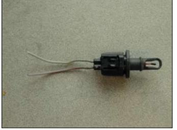
I. Strip off the wire loom from the sensor.
