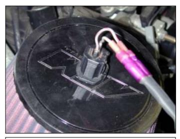
t. Insert IAT into the air filter end and attach to air horn.
