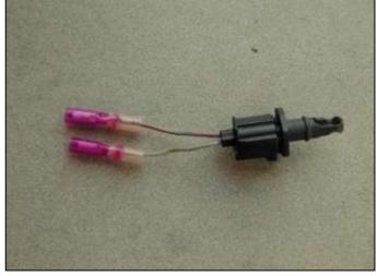
m. Strip a  $\frac{3}{4}$ " section off each end and attach the male bullet connector. Crimp carefully. For best results crimp at the seam.
