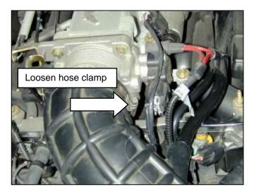
a. Loosen the hose clamp on the inlet air tube on the throttle body.
