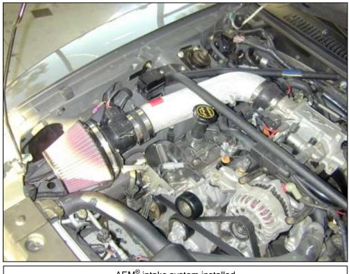
AEM<sup>®</sup> intake system installed
