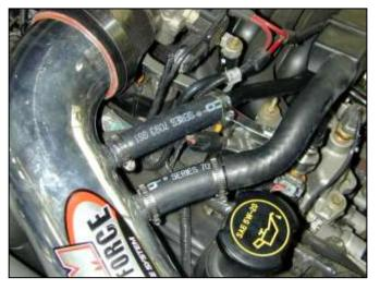
e. Attach provided 3/4" breather hose for the PCV and secure with provided hose clamps.
