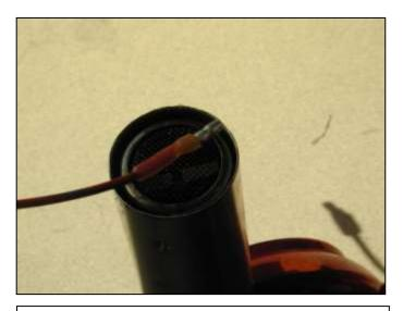
n. Heat each end of the connectors from prior step until the shrink wrap is secure around the wire.
