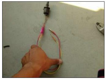
q. Match the solid gray wire from the IAT sensor female end and attach the solid gray wire male end connector. Do the same with the gray/red wire.
