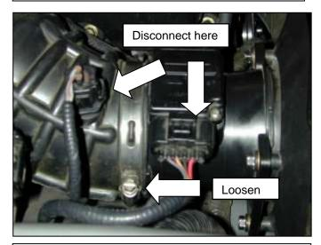
c. Disconnect MAF and IAT sensor connectors. Loosen hose clamp and remove inlet air tube.
