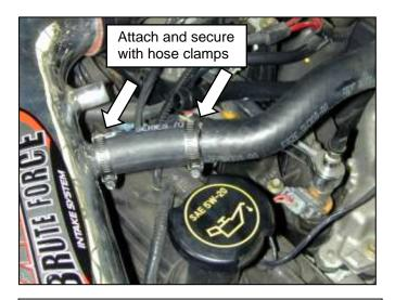
d. Attach the provided 5/8" hose for the IAC and secure with provided hose clamps.
