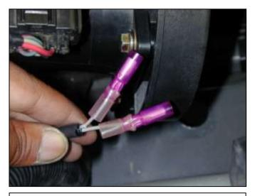
p. Strip off a  $\frac{3}{4}$ " section from each end and attach the 2 female end butt-connectors. Crimp and apply heat to each.
