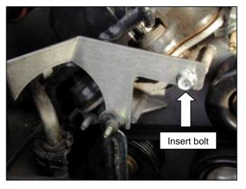
i. Attach bracket as shown with provided bolt. The slot on the bracket should be between the washer and the stock bracket.
