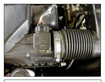
d. Remove the two screws retaining the MAF sensor and set them aside in a safe area. They will be installed with the  $\mathsf{AEM}^{\otimes}$  intake system.
