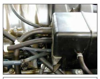
f. Remove the three hoses from the resonator chamber on the stock system. Some models have only two hoses and one vacuum cap to remove.
