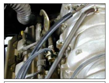
h. Install the 5/32" new hose on the fuel pressure regulator. Install the new 3/8" hose on the end of the exposed tube from the removal of the stock intake system if applicable. Use the 3/4 hose clamp to secure in place.
