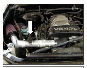
m. Install the MAF sensor in the inlet pipe using the stock mounting screws.
