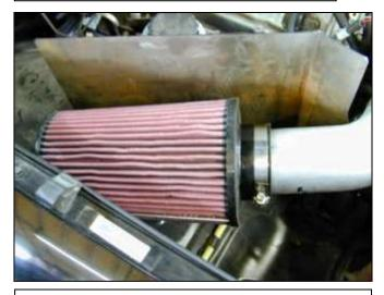
I. Install the air filter onto the end of the intake pipe and secure in place using the supplied hose clamp.
