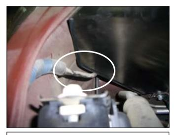
e. Relocate the stock wiring harness to the lower portion of the heat shield making sure it is free and clear.
