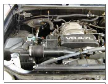
a. Stock air box system installed in vehicle.
