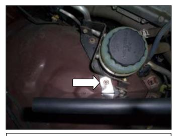
c. Install the heat shield mounting tab and use the stock nut to secure in place.
