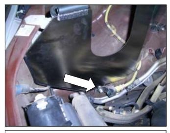
d. Remove the bolt securing the stock mounting tab. Insert the heat shield in place and use the stock bolt to secure in place.
