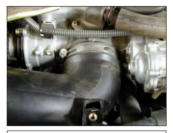
g. Loosen the hose clamp retaining the stock intake piping.
