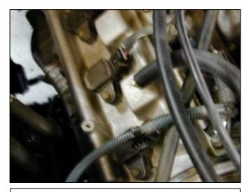
i. Install the new 1/2 hose and secure in place using one of the 1" hose clamps.
