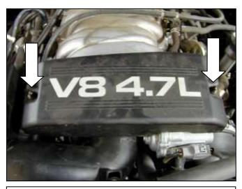
b. Remove the two nuts retaining the stock engine cover and remove.
