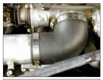
f. Install the rubber coupler on the throttle body and use the supplied #52 hose clamp to secure in place. Install the intake pipe in the other end of the rubber connector and secure in place using the supplied #48 hose clamp.
