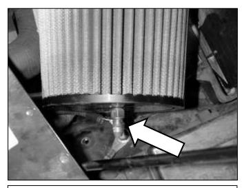
f. Attach the air filter element to the end of the inlet pipe. Insert the IAT into the air filter. Make sure the sensor is snug.
