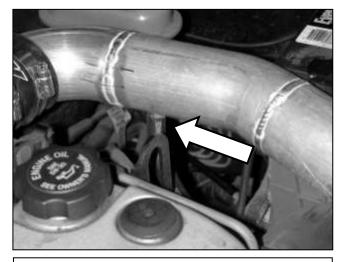
d. Attach breather hose to inlet pipe with provided clamp.
