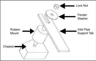
Proper installation of rubber mount assembly.
