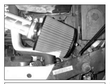
h. Ensure there is enough clearance around the air filter. Once proper fitment is achieved secure the air filter. Secure the intake bracket to the rubber mount installed in step 3c with a washer and nyloc nut. Refer to diagram for proper installation of rubber mount assembly.
