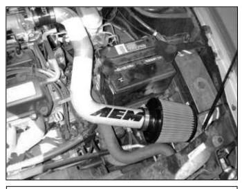
AEM<sup>®</sup> intake system installed
