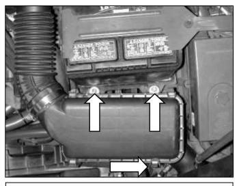
b. Remove the 3 bolts holding down the air box. Remove hose to the air box assembly.
