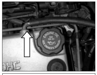
e. Attach breather hose to crank case with provided clamp.
