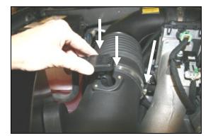
12. Re-position the factory intake tube onto the Airaid tube, and tighten the hose clamp. Next reinstall the Mass Air Flow sensor into the Airaid tube <u>using the two provided Button Head</u> <u>screws (#8)</u>. <u>Do not use the factory screws!</u> Do not over tighten!
