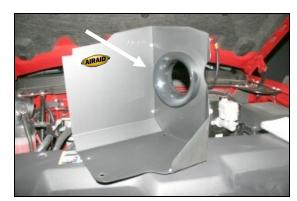
9. Assemble the Cool Air Dam panels (CAD) (#2 & #3) using five 6-32 x 5/16" screws (#10), #6 flat washers (#11), and 6-32 keps nuts (#12). Next install the air filter adapter (#5) into the panels as shown using three 1/4 - 20 x 1/2" button head bolts (#13), and 1/4" flat washers (#14). Apply the Airaid Decal as shown.
