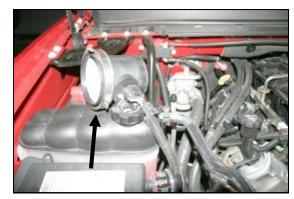
**6.** Remove, and set aside the **MAF** sensor from the factory airbox using caution to retain the factory clamp and seal.
