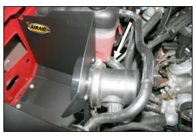
**11.** Reinstall the **MAF** sensor onto the filter adapter, and tighten the clamp.
