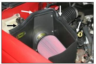
**9.** Install the Airaid Premium Filter (#1) onto the Airaid intake tube as shown, and then tighten the hose clamp. Next, install the weather strip on top of the **CAD**, starting at the right fender working your way towards the front of the vehicle.
