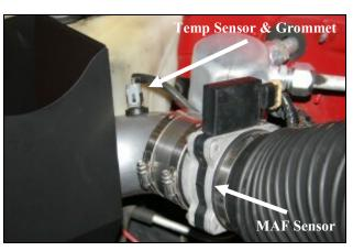
**8.** Connect the **MAF** sensor to the stainless steel coupler and tighten the hose clamp. Install the factory grommet removed in step #1, into the hole in the Airaid intake tube. <u>VERY CAREFULLY</u> install the factory temperature sensor into the grommet.
