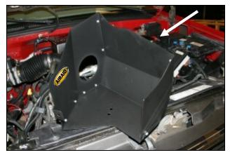
**3.** Assemble the three Cold Air Dam (CAD) panels (#s 2, 3, &4) as shown using nine 6-32 screws (#8), nine #6 washers (#7), and nine nuts (#9). Apply the Airaid Foil Decal onto the Panel as shown.
