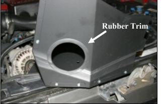
**4.** Install the supplied rubber trim (#15) into the hole in the **MAF** Panel (#2) as shown.
