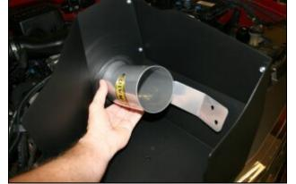
5. Insert the air intake tube that was removed in step #1 thru the hole in the **MAF** panel and then rotate it clockwise so that the holes in the bracket on the tube line up with the two holes in the bottom panel.
