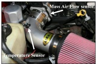
1. **Disconnect the negative battery cable.** VERY CAREFULLY! Remove the air intake temperature sensor first, and then the grommet from the air intake tube and set them aside. .
