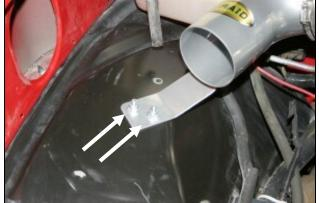
**2.** Remove the two nuts and washers from the bolts that secure the air intake tube to the inner fender. Save the 3" x 2" plate from the bottom of the fender for reinstallation in step #7. Remove the intake tube from the vehicle.
