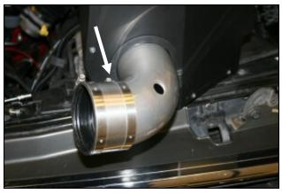
**6.** Install the stainless steel coupler removed in step #1 onto the air intake tube and tighten *only* the hose clamp on the tube.
