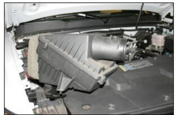
**3.** Rock the factory airbox back and forth while lifting up on it, and remove it from the vehicle. It is only held in place by grommets.
