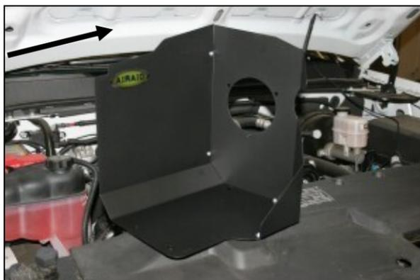
**5.** Assemble the two Cold Air Dam (CAD) panels (#2 & #3) using five 6-32 Phillips screws (#6) five flat washers (#7), and five keps nuts (#8) as shown. Make sure that panel #2 is located inside of panel #3. Apply the Airaid Foil Decal onto the Panel as shown.
