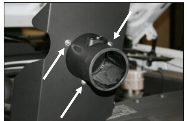
**6.** Install the filter adapter into panel #3 as shown, using three 1/4-20 x 1/2" button head bolts (#10), and three flat washers (#11).
