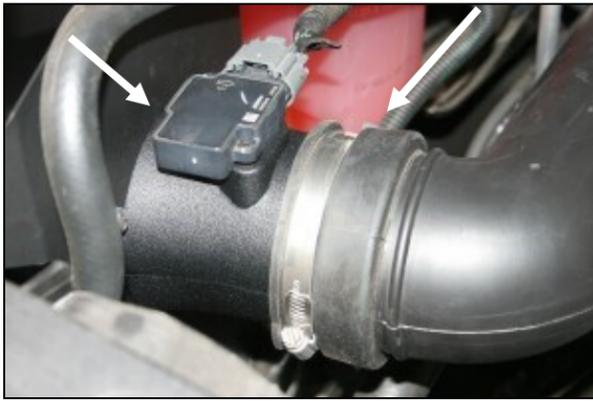
8. Reinstall the MAF sensor onto the filter adapter using two 8-32 x 5/8" button head screws (#9). **Do Not Use The Factory Screws!** Reconnect the factory air intake tube to the filter adapter and tighten the hose clamp.
