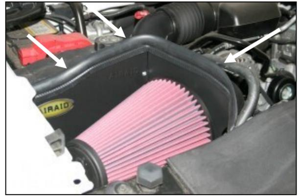
9. Install the Airaid Premium Filter (#1) onto the filter adapter and tighten the hose clamp. Next install the weather strip (#5) onto the top of the CAD as shown. Start at the right fender and work your way around towards the radiator.
